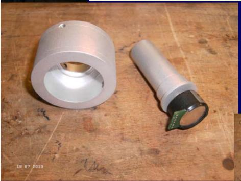
For easy assembling the collet is made of two aluminium parts
