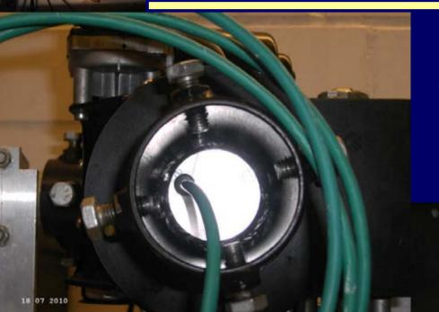
As there is not space enough for the AZ encoder inside the rotator, a special collet was made on a lathe, which finds its
