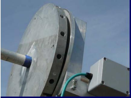
The central hub consists of 2 solid plates, which are rotatable against each other, this enables us to fix the aluminum tubes and inserting the meshes at ground level
