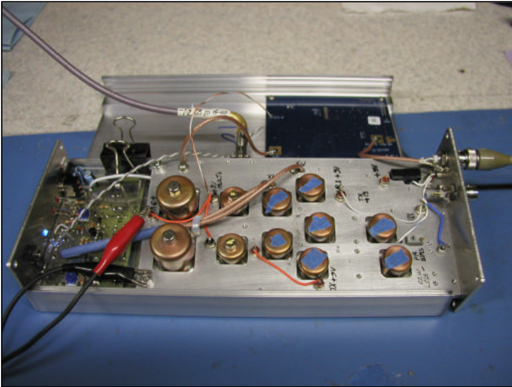
Testing LO and Mixer with lab GPS.
