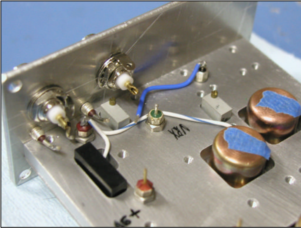
Holes from PCB to substrate tapped and feed-thru capacitors installed.
