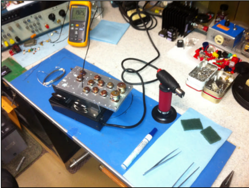
Preheating aluminum substrate and PCB to 190F facilitates quickly soldering pipe caps.
