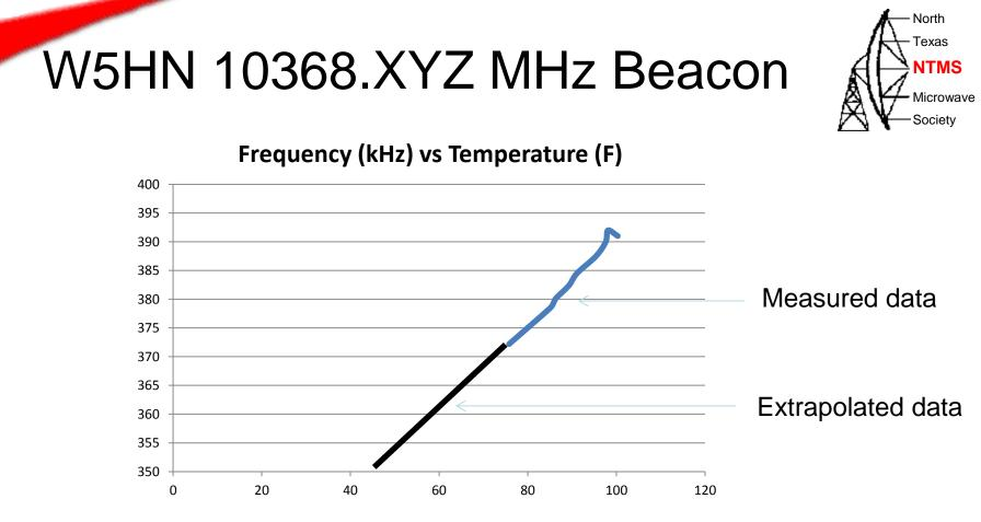
DB6NT specs the unit at 5ppm which equates to about 52 kHz at 10368 MHz I chatted with Steve N5AC about setting up a VHF Apollo board at 108.004 MHz which when multiplied times 96 = 10368.384 MHz. Concerns are spurs and how to key and ID the beacon...Thoughts and ideas?? Steve will look at options and send us a board to evaluate.
