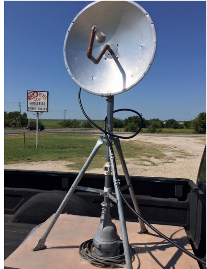
2 ft prime focus dish in bed of truck
