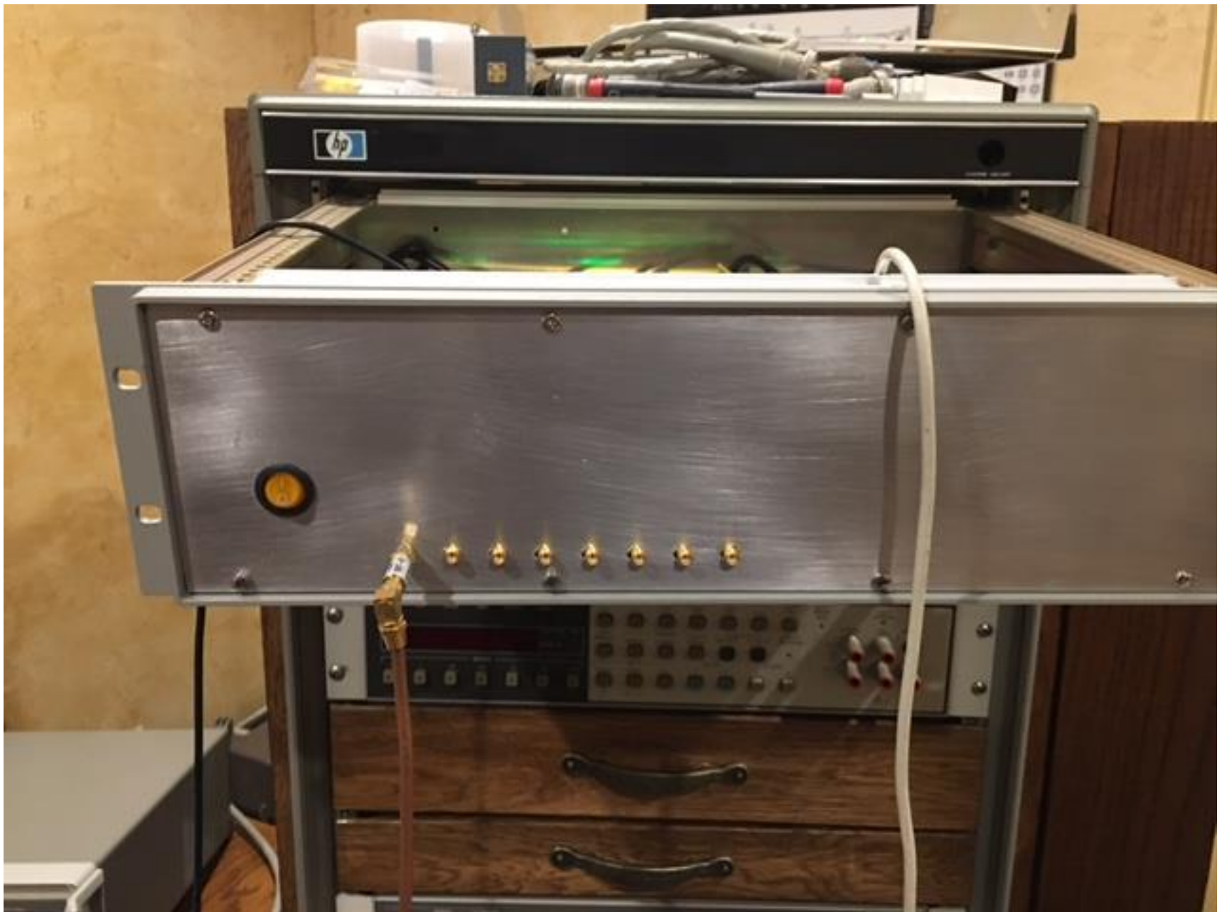
The unit mounted in a rack box with 3 power supplies; 12V GPS, 6V, Eval Board, 3.3 V Reference Oscillator interface. The cable is USB connection to computer.
