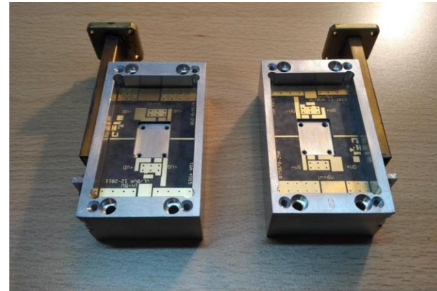
Atu box with PCCB for SSPA with TGA4915CP
