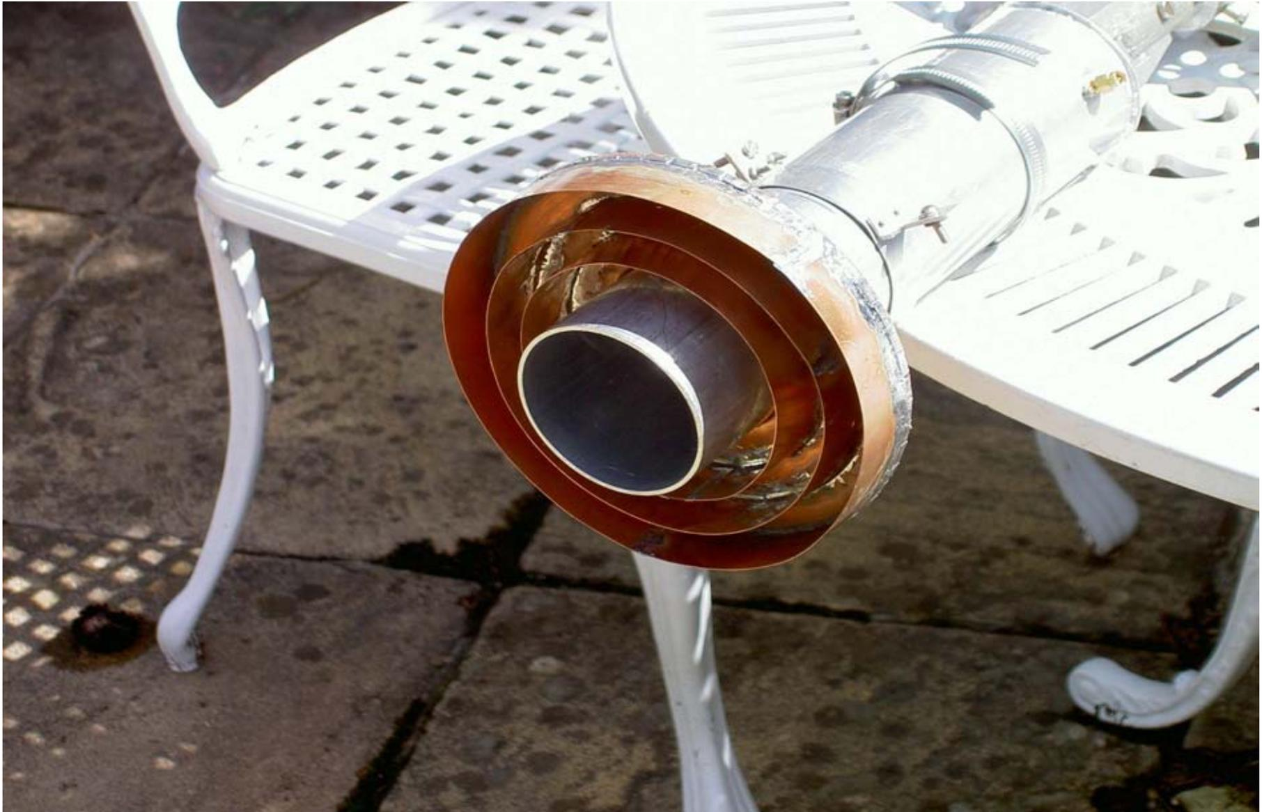
VK3NX Septum feed scaled from RA3AQ design, see [www.ok1dfc.com/eme/technic/septum/ra3aq-23cm04fd.pdf](http://www.ok1dfc.com/eme/technic/septum/ra3aq-23cm04fd.pdf)
