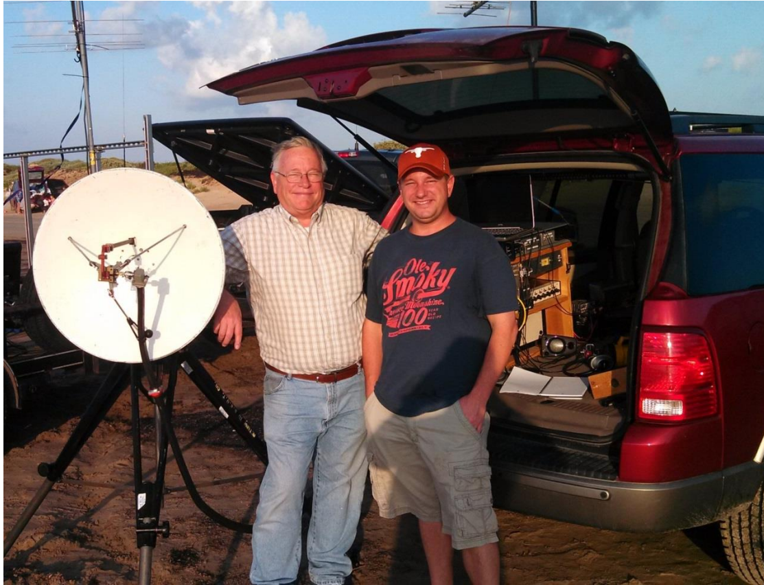
Flex-1500, DEMI xvtr and 25 watt TWT and 27 dBi 2 ft Dish Antenna – Best DX 180 miles
