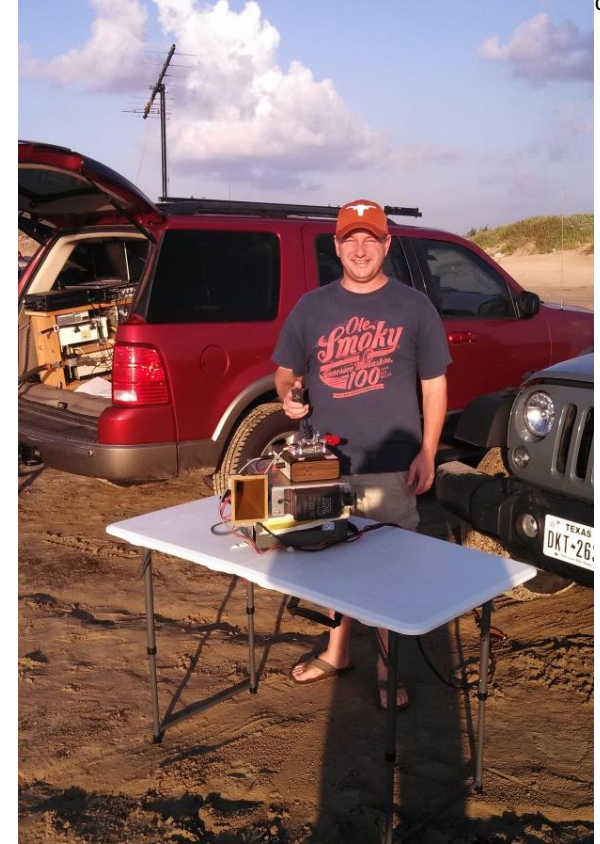
IC-271A, HB 3 watt Transverter and 15 dBi Horn Antenna – Best DX 180 miles
