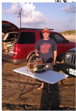
IC-271A, HB 3 watt Transverter and 15 dBi Horn Antenna – Best DX 180 miles
