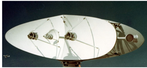
2-18 GHz High Gain Airborne Direction Finder
