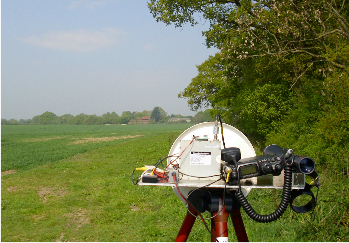
The transverter in action – yes I forgot about having to plug the microphone into the FT817!
