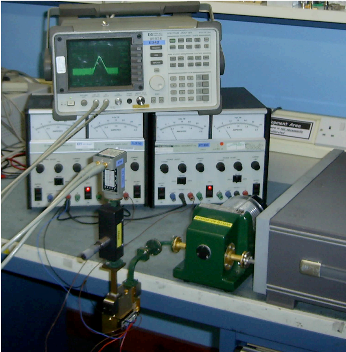
Test set-up shown measurement 40 - 48GHz, 47.088GHz on screen. This used a Wiltron 40 -60GHz generator and a Flann attenuator and transition WR-19 to WR-28. On the output side a transition to WR-22 and WR-22 attenuator fixed at 40dB and a 33-50GHz HP harmonic mixer with HP 8563E analyser. I later checked the 28 - 40GHz response using a Spacek doubler on my sig gen, and an MI power meter.
