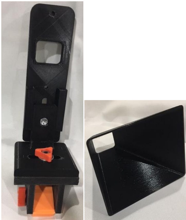
KOXL version of 3-axis receiver mount and light shield
