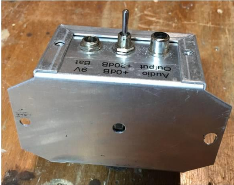
Receiver box, from left to right: 9V battery plug, gain boost switch, and audio output
