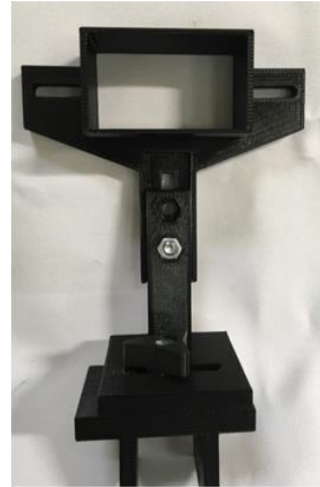
Vertical slider w/light shield Horizontal slider Tripod base mount Fully assembled
