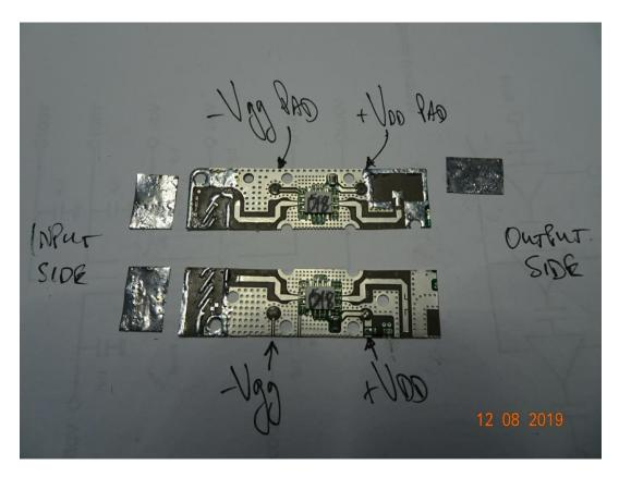
To maximise adhesion of the "tinned" copper shim material, on the Input I chose to leave all the RF Tracks intact.
