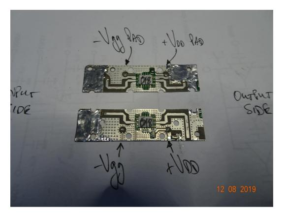
Readers will hopefully note that I have restored (created) the PCB Mounting holes. I suggest 8 holes are needed for best RF Grounding. I cannot emphasise enough how important it is to fit all 8 Screws (3mm ?) or Self Tappers to ensure best RF Grounding. Poor RF Grounding means reduced Output !!!
