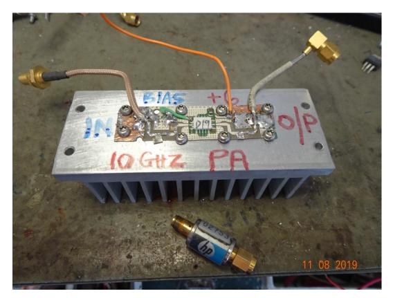
This Amplifier requires 2 Supply Rails... a Negative Bias Rail Vgg (Green wire) of circa -0.20 Volts and +VDD Rail in the range +5 to +6 Volts maximum.
