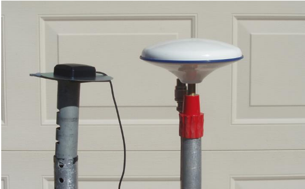
Fig 8: The u-blox kit comes with two consumer grade antennas and a ground plane as shown on the left. On the right is a survey grade antenna which we have used for our testing.
