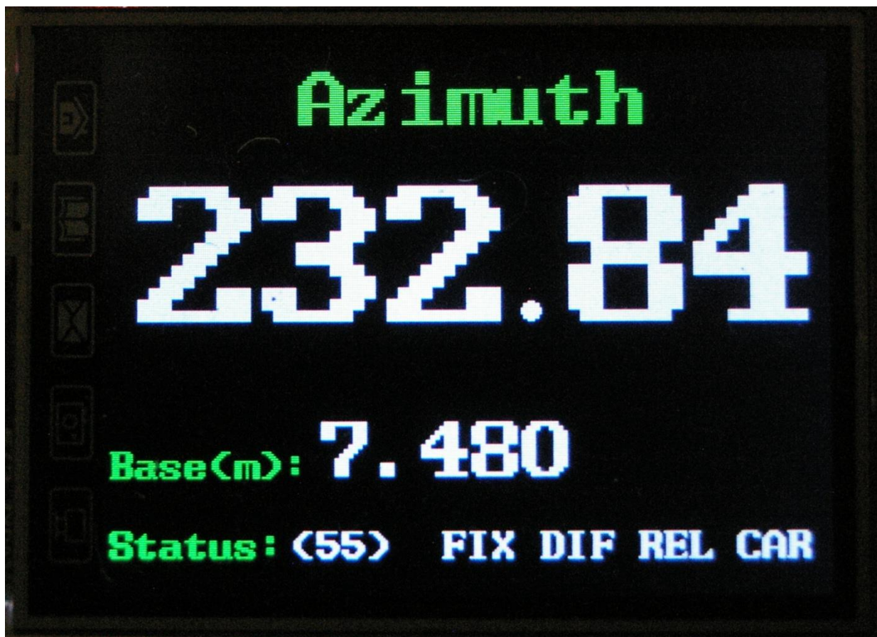
Fig 3: This display mode shows the Azimuth (232.84 Degrees in this case), The length of the base between the two antennas (in this case 7.480 meters) and the Status (in this case 55) in brackets which indicates the bearing derives from a Carrier Phase measurement which gives the accuracy we require.
