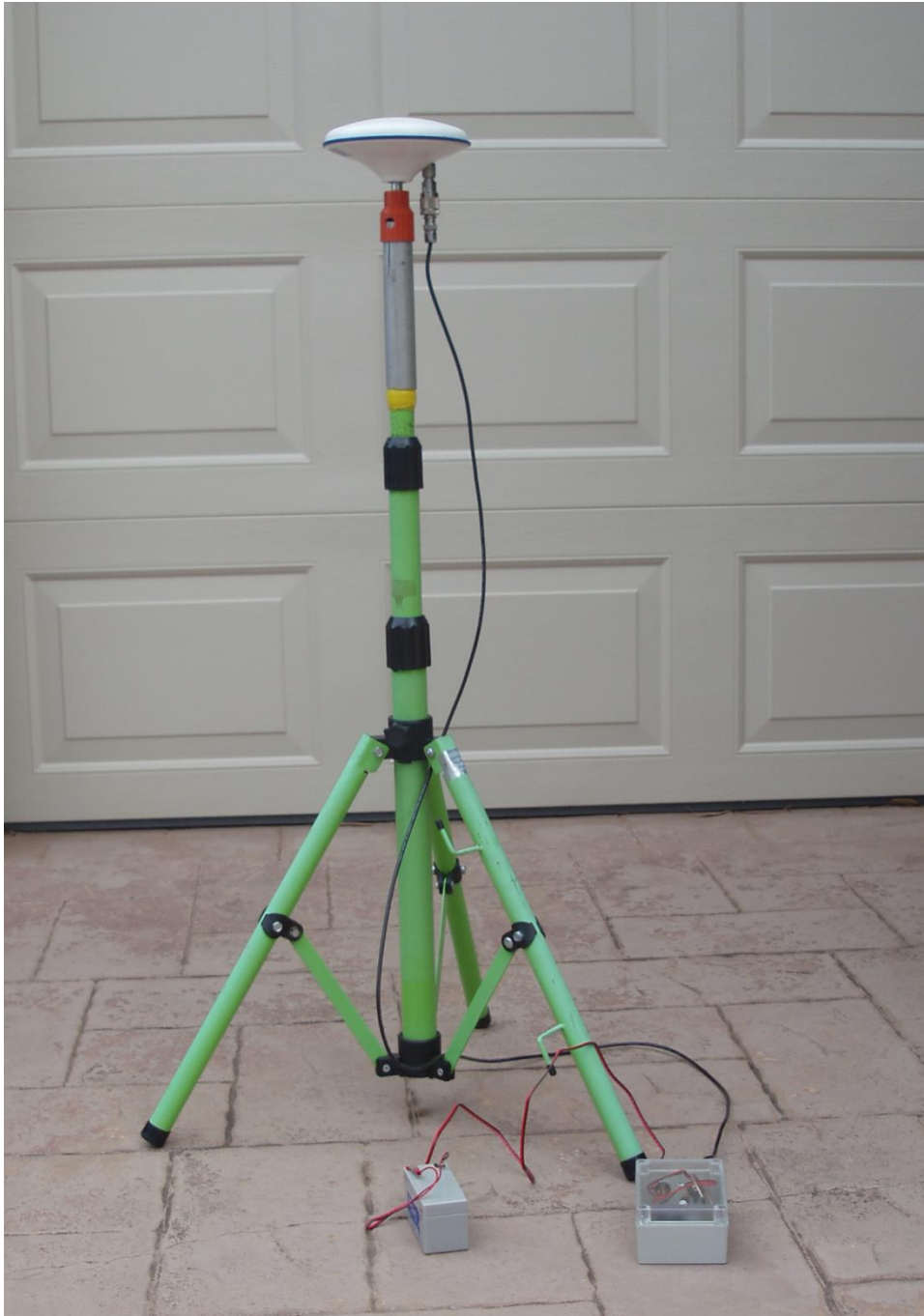
Fig 7: Base antenna with u-blox evaluation board in weather proof box and separate battery
