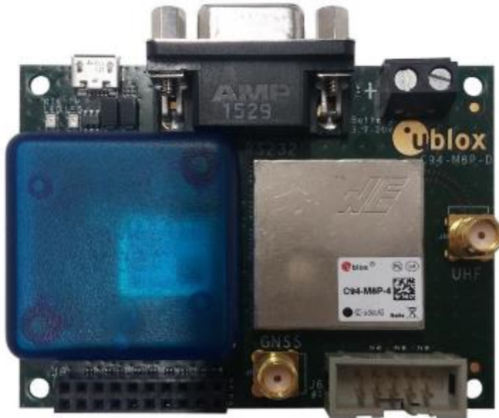
Fig 5: u-blox Evaluation Board - two identical boards come with Evaluation kit as well as cables and both GPS and UHF antennas. GPS unit under blue cover and VHF link under metal cover.
