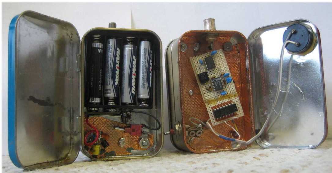
Figure 1 Circuitry and batteries built into a pair of Altoids tins
