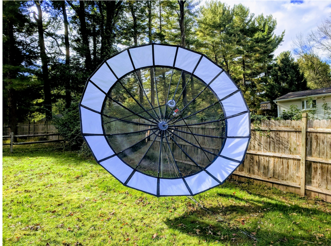
Completed 4m dish with completed stress extension.
