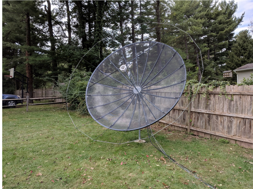
3m dish with 4m framework – no Mylar covering.
