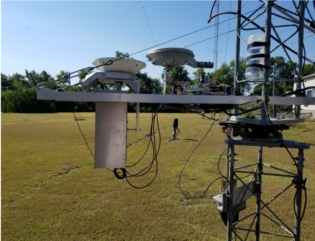
Figure 4. Equipment platform with both 77 GHz and 47 GHz transverters mounted
