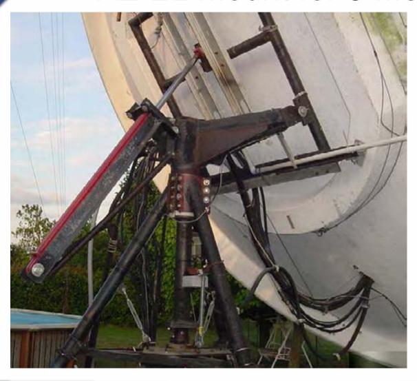
Hydraulics for elevation drive
