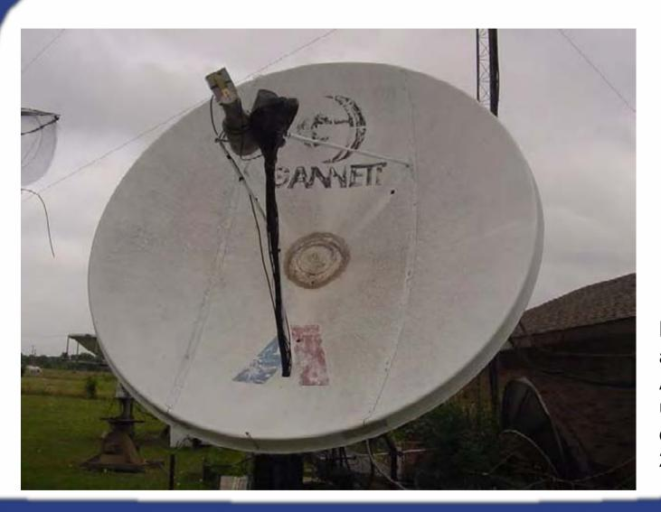
Used for EME on 902 MHz 1296 MHz 2304 MHz 3456 MHz 5760 MHz 10368 MHz
