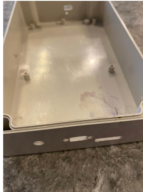
Openings for power switch, recharge port and SD card interface slot
