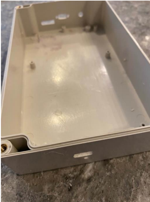
Opening for PME280 sensor and standoff mounting hole
