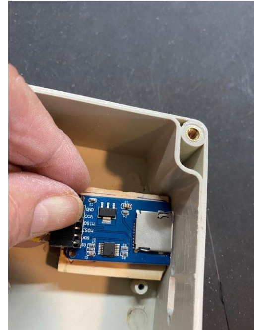
Mount SD card on scrape wood riser, trim front edge of SD card interface PCB
