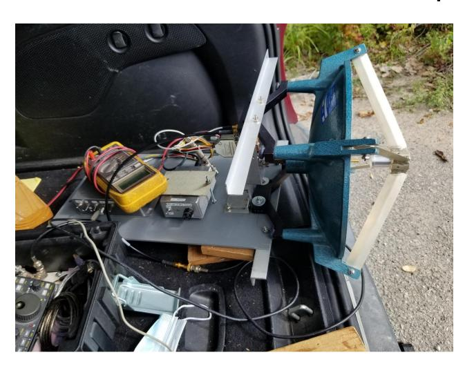
This is not the way to aim an antenna with a .5 degree 3 dB beamwidth!
