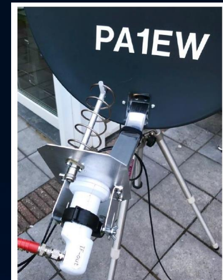
Figure 2: Completed dual-band feed – July 2019
