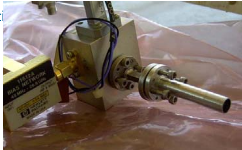
Feed Installed on Mixer
