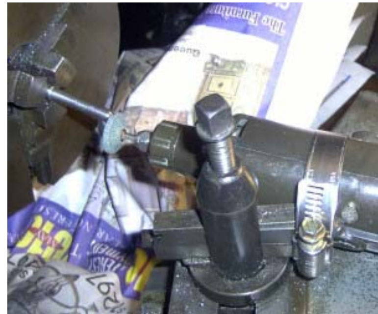
Temporary "Tool Post" Grinder
