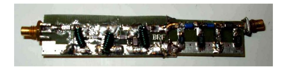
With mod amp 10dBm in at 10MHz gave 13.8dBm at 90MHz.
