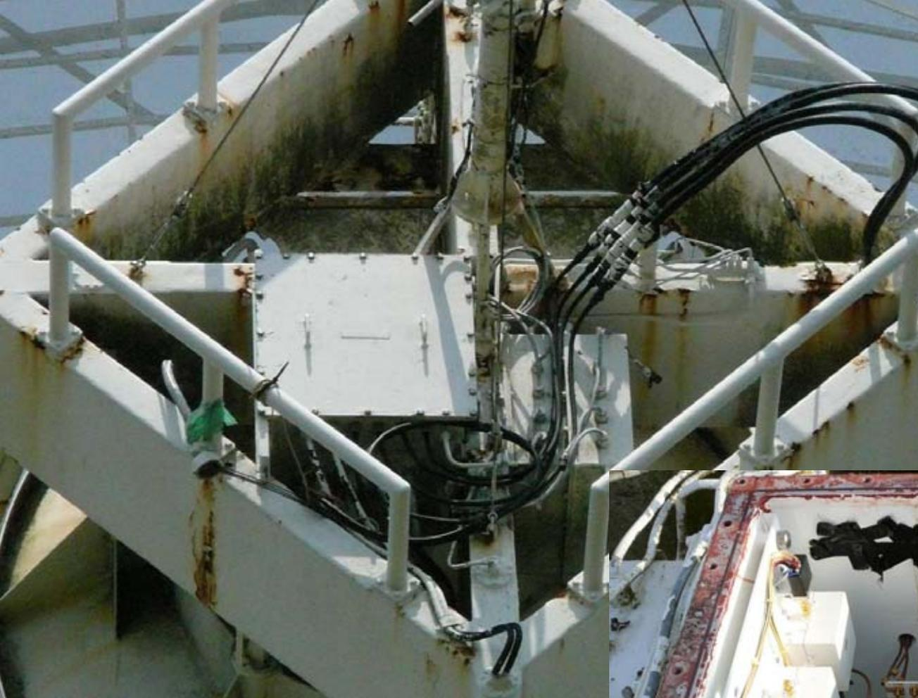
1st LNAs were installed in the metal box behind the sub-reflector.
