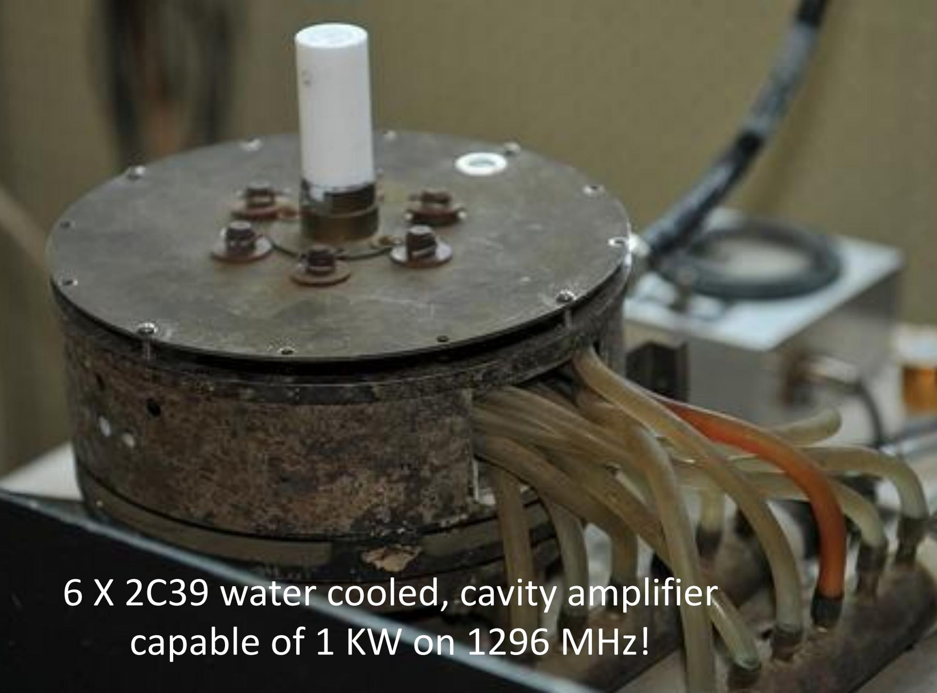
6 X 2C39 water cooled, cavity amplifier
