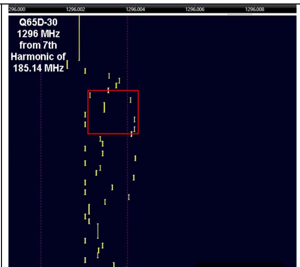
Figure 13. Correct tone bandwidth (1733 Hz) at 1296 MHz for Q65D-30 by using 7 th harmonic of 185.14 MHz.
