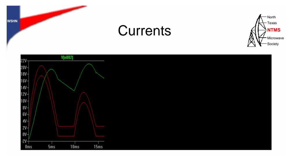
Peak diode currents 60+amps, 100 amps turn on.... Limited by Resistance of Capacitors.
