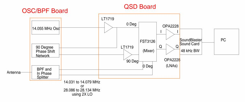
Quadrature Sampling Detector with in-phase feed of the RF and quadrature feed of the LO and 2 low noise IF amplifiers that provide I&Q for the sound card.
