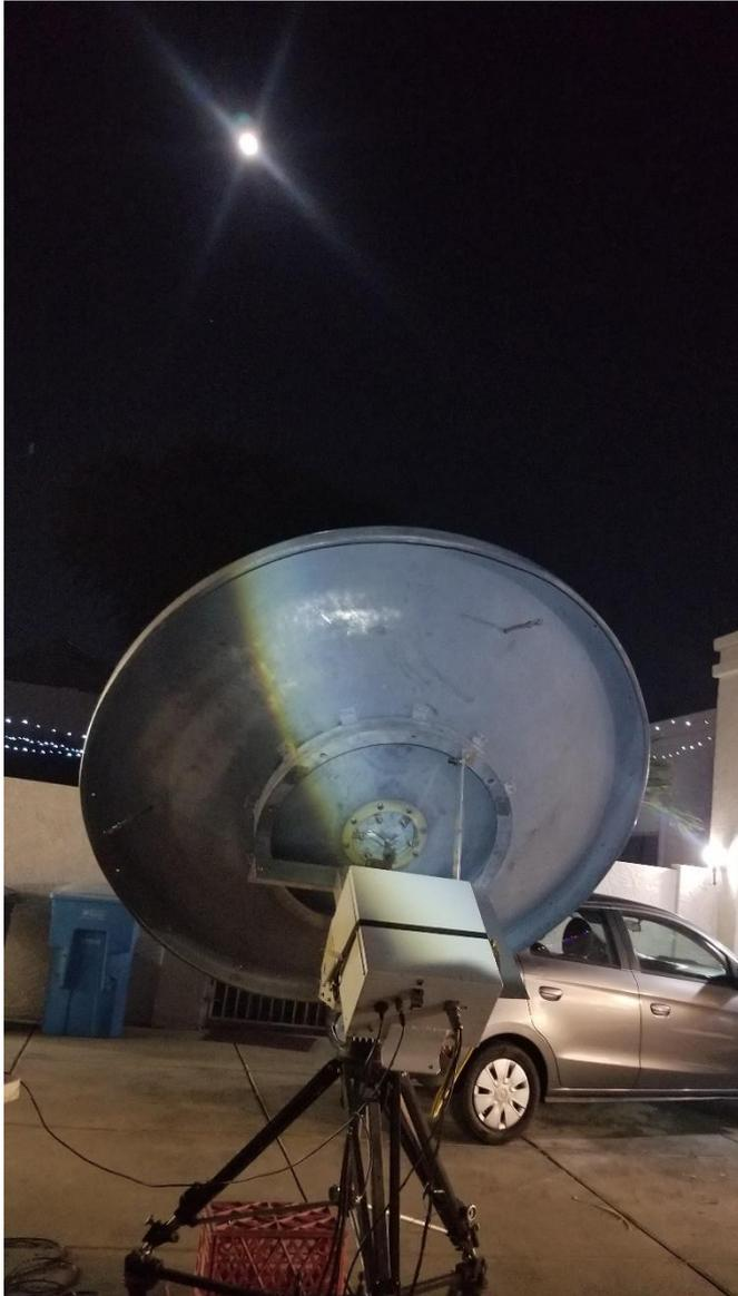
5<sup>th</sup> Generation Roll Around station using the 6ft dish and a 60W Solid State Amplifier listening to EME from the German Beacon DL0SHF
