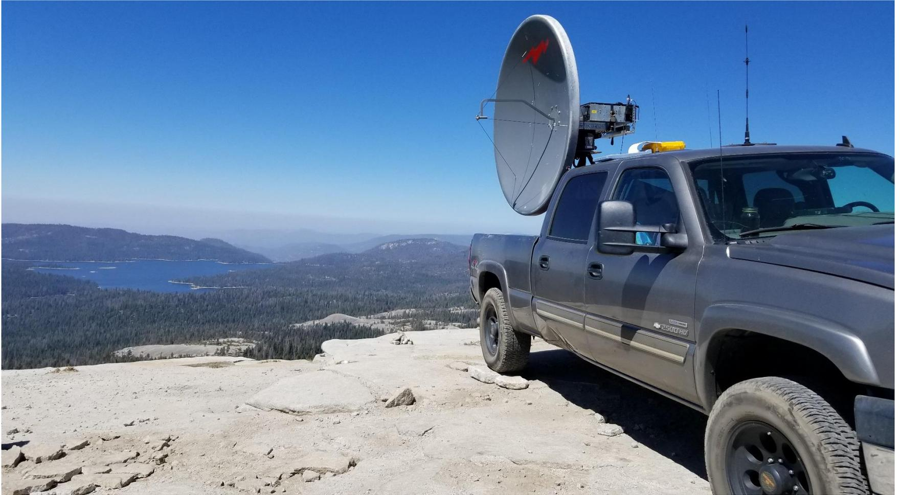
4<sup>th</sup> Generation Truck Mounted AD7OI station using the 6ft dish and a 50W TWT. Total EIRP = 1.02 MW From Bald Mountain Lookout above Shave Lake, Ca. Elev 7730 feet
