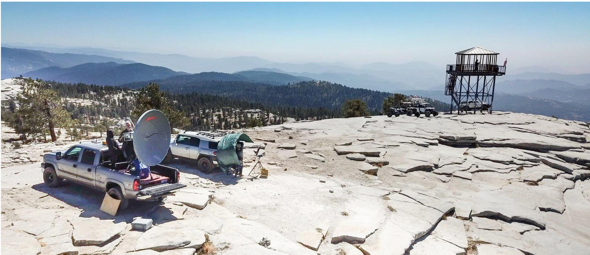
Latest AD7OI portable station using the 6ft dish and a 50W TWT rig. Total EIRP = 1.02 MW
