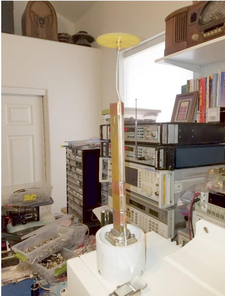
10 GHz Slotted Waveguide Antenna and WA5VJB
