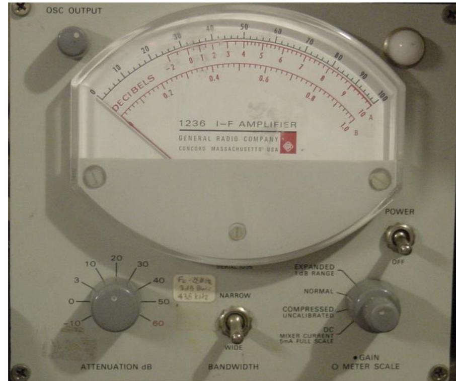
These meters provide a 30 MHz IF amplifier with up to several MHz of bandwidth which makes it easy to measure sun and moon noise – they can be easily retuned for 28 MHz
