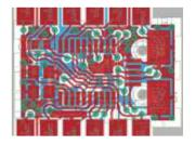
A programmable crystal replacement. It has three independent outputs with frequency range 3.5kHz to approx 300MHz, and can be optionally GPS disciplined. Configuration is by a micro-USB connector and PC terminal emulator
