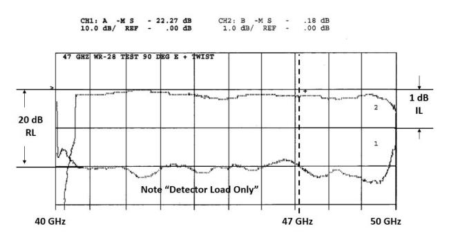
Figure 10 Rigid Waveguide E Plane Bend + Twist
