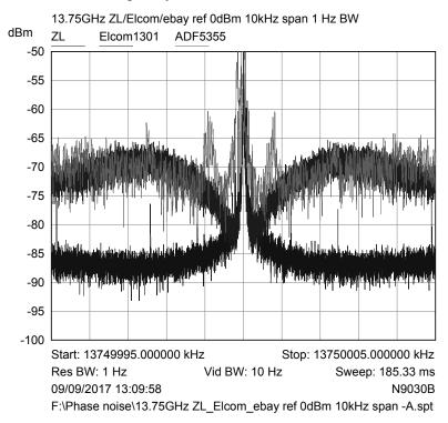
Comparison of ebay ADF5355 board with Elcom 1301 and ZL 14G synthesisers
