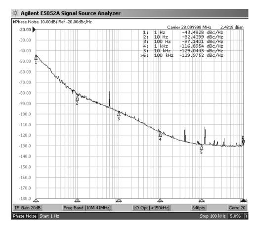
ICOM-7300 Phase Noise 28.1MHz 20% power output CW. This plot extends from 1Hz to 100kHz.
