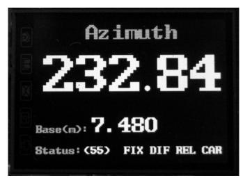
Fig 3: This display mode shows the Azimuth (232.84 Degrees in this case), The length of the base between the two antennas (in this case 7.480 meters) and the Status (in this case 55) in brackets which indicates the bearing derives from a Carrier Phase measurement which gives the accuracy we require.
