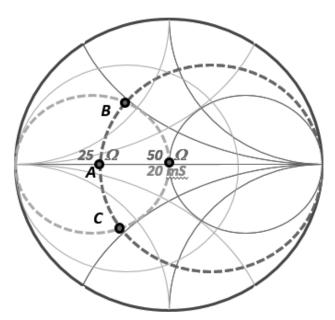
Figure 8 Lumped element matching
