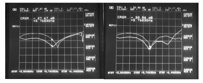
First Sweep: RL = 27 dB, ISO = 19 dB Best Adjustments: RL = 30 dB, ISO = 28 dB
