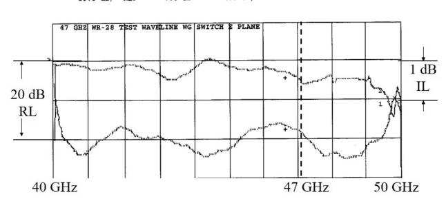
CH1: A -M S - 18.87 dB CH2: B -M S - .57 dB 10.0 dB/ REF - .00 dB 1.0 dB/ REF - .00 dB
