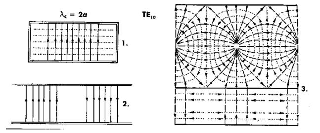
Figure 2 TE<sub>10</sub> Propagation Mode (Cut-off Frequency = 21.1 GHz)
