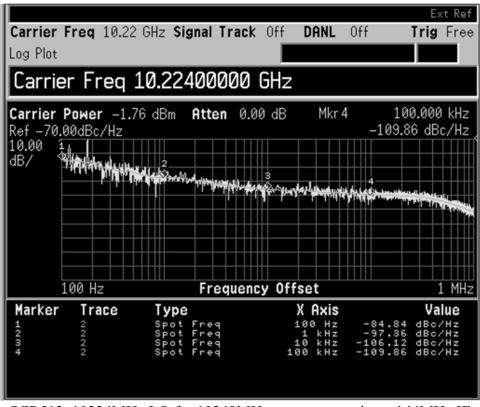
SCR513 10224MHz LO for 10368MHz transverter using a 144MHz IF
