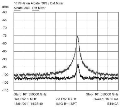
The plot shows the oscillator on 161GHz. The higher (blue) trace was measured with a commercial mixer (110-170GHz), the lower used a 'test module' from an Alcatel 38GHz 'white box'. This shows that even at 160GHz the test modules work as a low cost mixer! The signal bandwidth is much greater than the spectrum analyzer 2MHz bandwidth, so the true power is greater than the plot.
