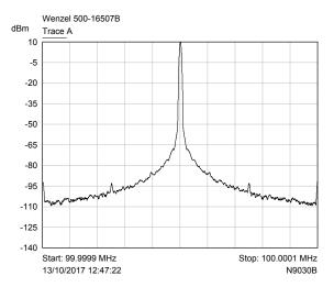
Noise in dB/Hz 200Hz span. Spurs at 50/100Hz are pickup on the bench. Ignoring those noise measured is circa -120 dBc/Hz down on the fundamental at +/- 100Hz.
