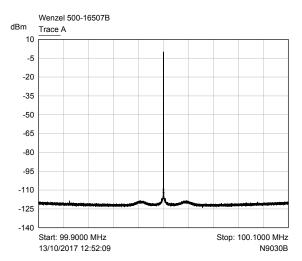
Noise as measured in dB/Hz with 200kHz span, note reference is +10dBm so wideband noise displayed is circa -130dBc/Hz, this is limited by analyser noise performance
