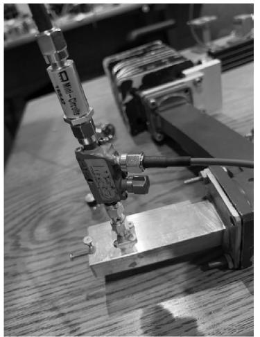
Setup with converter dummy load and directional coupler. Figure 6
