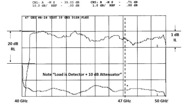
Figure 8 39 GHz Dish Flex Waveguide with 90 degree H Plane bend
