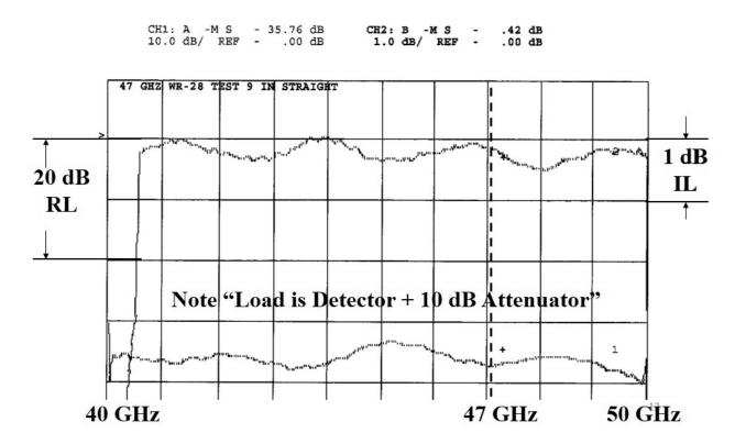
Figure 6 9 inch (23cm) Straight Waveguide
