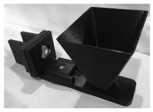
Fully assembled K0XL 3-axis receiver mount with attached light shield
