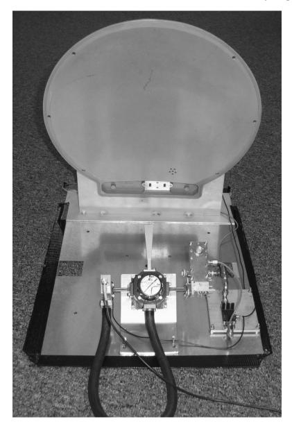
The idea of putting together a quick transverter for 47GHz came to me after 2012 RAL. Having come away with an offset dish (thanks Peter), and a WR-28 four port waveguide switch. It was decided to try and put something together in 4 hours, and have it ready for the '76<sup>th</sup>' August tests. Of course it took 6 - 7 hours to build, but was finished in time!
