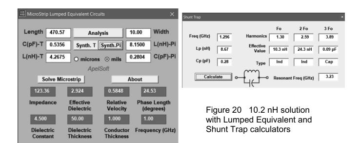
In summary, the output match is comprised of a 246 mil long x 40 mil wide trace, a shunt 0805 2.4 pF chip cap to ground, followed by a series 0805 4 pF capacitor and a shunt 470 mil x 10 mil transmission line to ground through a 35 mil via (total approximates 10.3 nH). The RF
