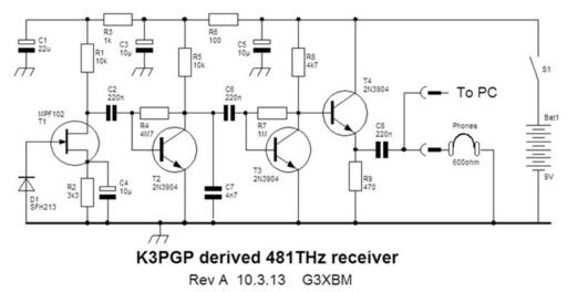
I made a couple of parts modifications. I used a BPW34 detector instead of the SFH213, I also replaced the MPF102 JFET with a 2N5457, and used a 1 meg resistor on the base of T2 instead
