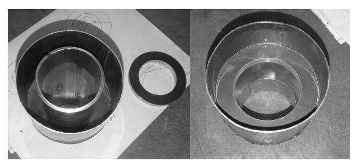
With a special ring lathed from aluminum and placed inside the launcher section, it held the funnel centered and clamped on the main copper pipe waveguide. It was then soldered being held in place making it concentric or true.
