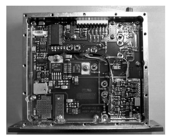
Reference / DC side of the synthesiser. The track at the extreme left of the reference TCXO upward carries the 10MHz signal. Connect into the capacitor at the top of the track when using an external 10MHz reference. Removing the +5V supply to the internal TCXO at the same time is probably a good move.
