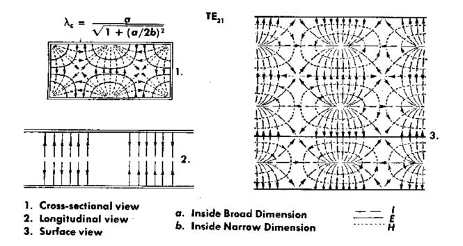
Figure 4 TE<sub>21</sub> Propagation Mode (Cut-off Frequency 59.6 GHz)
