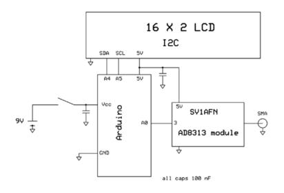
Figure 1. An Arduino reads the DC output voltage of the AD8313 logarithmic detector, then translates to dBm to be displayed on the serial LCD module.
