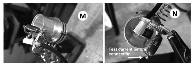
Remove the red (+) wire from the board and attach a current limiting resistor to the positive board pad and reattach the red (+) wire to the other end of the current limiting resistor (N).
