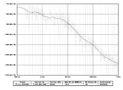
Phase Noise plot using KE5FX program
