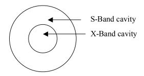
The inner cavity is a conventional open ended circular waveguide covering X-Band; the outer is coaxial waveguide covering S-Band.
