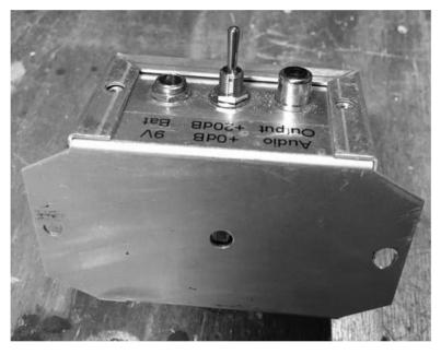
Receiver box, from left to right: 9V battery plug, gain boost switch, and audio output
