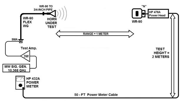
Feed Horn Test Equipment Setup
