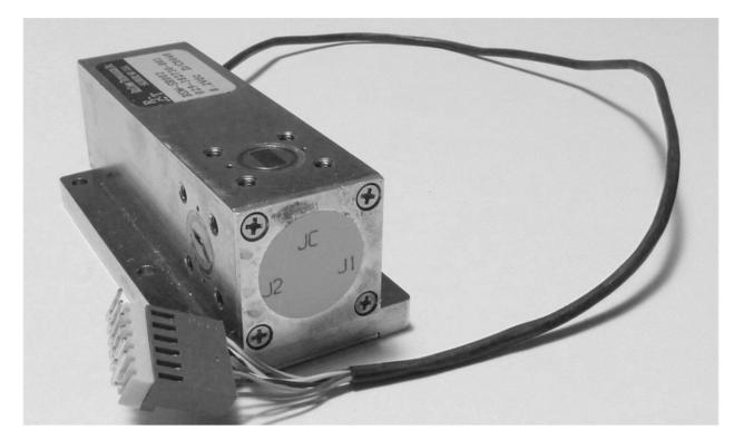
Figure 20 Relcomm Tech E Plane Waveguide Switch
