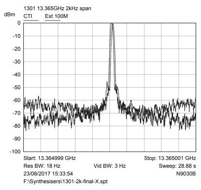
Comparison with +/- 1kHz span 18Hz BW
