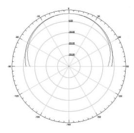
Figure 5. TE<sub>11</sub> Pattern produced by open-ended coaxial waveguide
