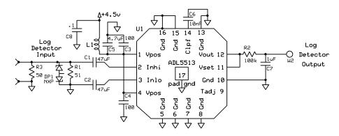
Figure 6 Front-end for Audible Field Strength Meter using 4 GHz ADL5513
