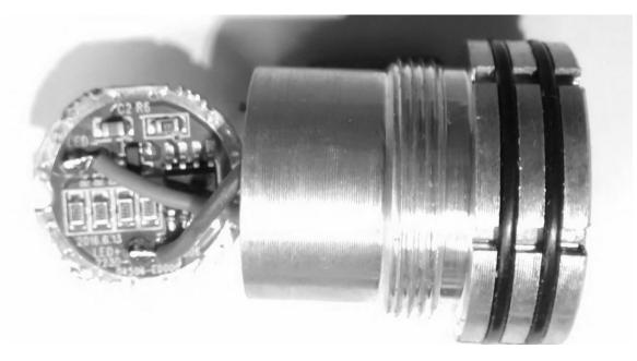
Figure 4 PCB Removed from LED Assembly
