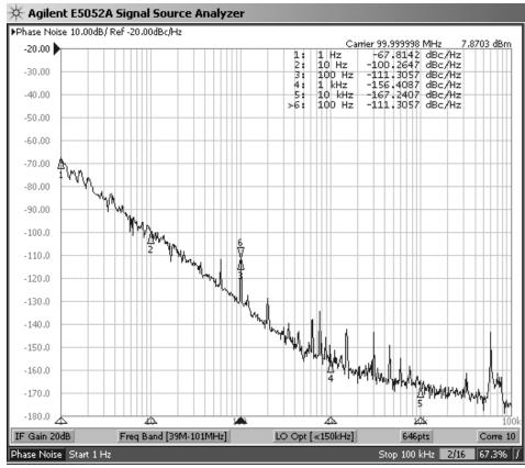
009 Plot 2 100MHz Wenzel Reference Oscillator locked to GPS 10MHz Reference Signal
