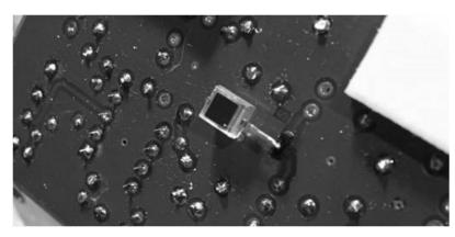
Close up view of the smd JFET and the BPW34 detector, the blob upper right is the double-sided mounting tape
