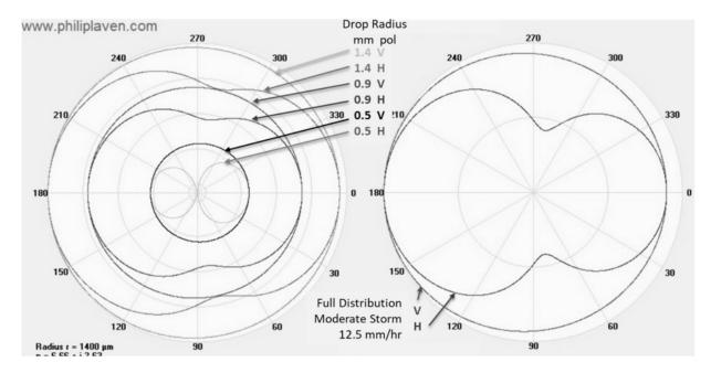
Figure 12. 24GHz plots of scattering. On left, three drop sizes in two polarizations. On the right, scattering with a drop size distribution as found in a moderate rain storm of 12.5mm/hr (1/2 inch/hr).
