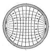
Figure 3. Electro-magnetic fields in circular waveguide for  $TE_{1,1}$  Mode
