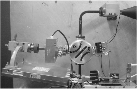
Waveguide switch in TX position
