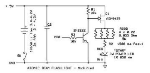
You'll need to remove the 3 pin smd device. After removing it, put a dab of solder on the 2 pads we'll use for 2N2222A transistor's collector pin (left pad) and emitter pin (lower right pad) (K), bend the base pin up to the back of the transistor (L).
