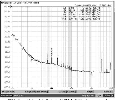
0013 Phase Noise plot of a typical 10MHz GPS reference signal used to lock a stations other oscillators.
