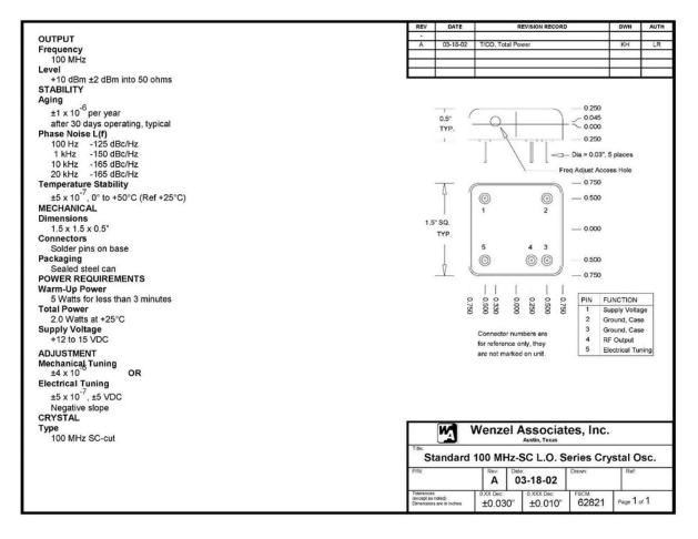
Specification as shown with the crystal as advertised. The 500-16507B supplied, had electrical tuning which I suspect is 0 to -5V. On frequency is approx. -2.0V.
