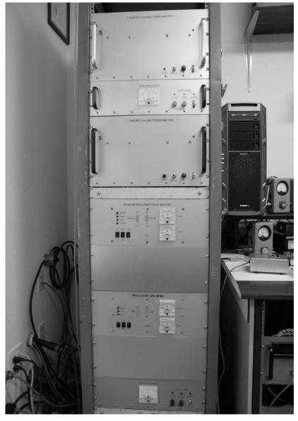
Figure 5 AA5C LDMOS KW Amplifier Rack
