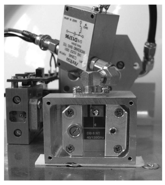
The harmonic mixer is a DB6NT pcb No.47. The case used is a 122GHz housing from Philipp DL2AM.
