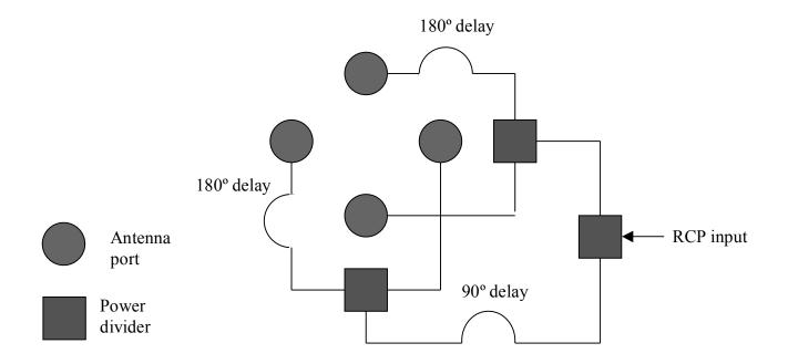
Figure 8. Network for producing circular polarization
