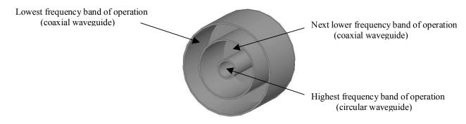
Figure 1. Coaxial feed configuration for multi-band operation
