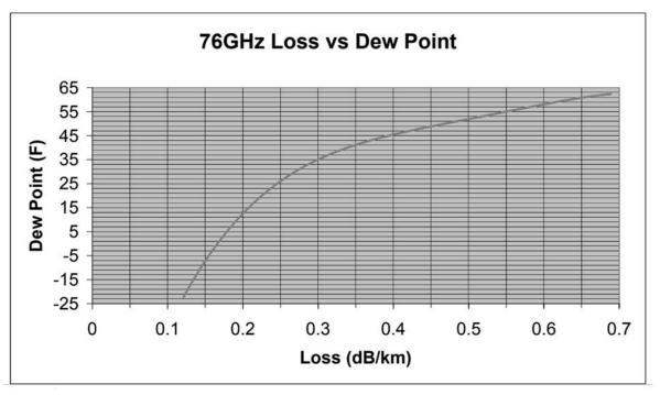
Figure 2 WA1ZMS Atmospheric Loss Chart for 75 GHz
