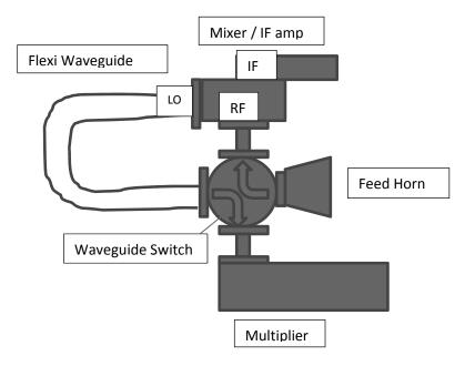
Waveguide Switch in Receive position.
