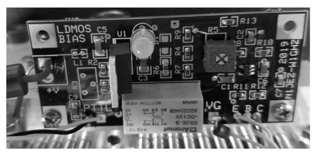
Figure 2 - LDMOS Bias Board Prototype mounted on amplifier
