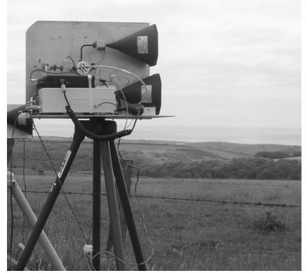
In Operation at Firle beacon with 10GHz transverter and FT817 fitted.
