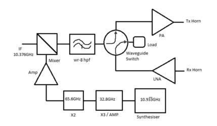
Transverter block diagram. Waveguide switch shown in TX position
