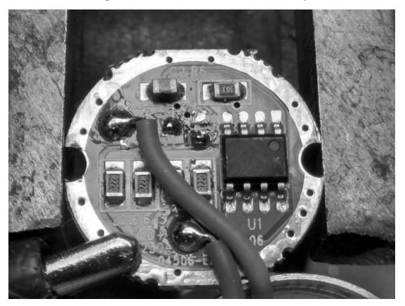
Figure 5 PCB with Surface Mount Part Removed
