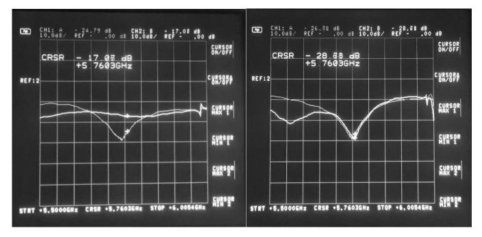
Once again it seemed the N connector was the answer. The pix on the left are the Return Loss and Isolation Sweep adjustment before the CP bolts were screwed in at all. The RL is around 24 dB and the Isolation at around only 17 dB, similar to the other feeds at this point.
