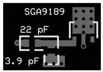
Figure 18 Input RF impedance match
