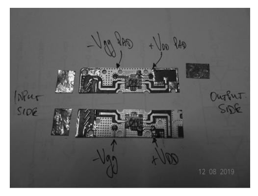
To maximise adhesion of the "tinned" copper shim material, on the Input I chose to leave all the RF Tracks intact. So... "tin" all surrounding copper tracks on the PCB and then lap the preformed shim over the entire surface and solder. Note also the I/O Striplines have been trimmed ready for their RF connections.
