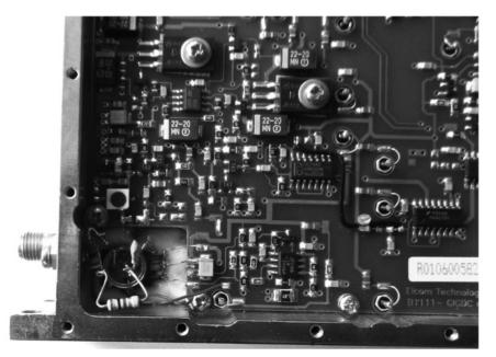
The modification of the DFS1301, was to add an SMA connector, connected to a 47 ohm load resistor. The SMA centre pin is then connected via a 100R and 1n0 capacitor to one end of the 100MHz crystal, removed from the collector of the oscillator.
