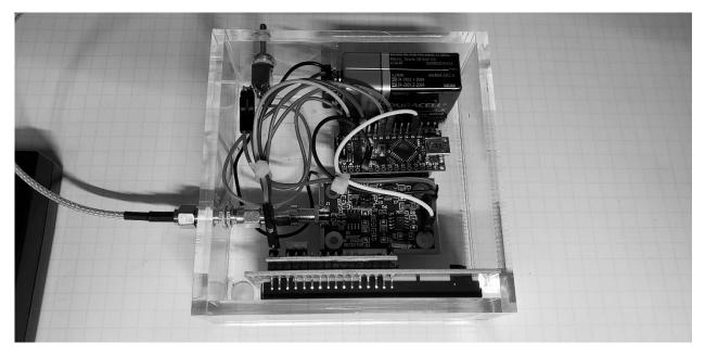
**Figure 2.** The LCD is spot glued to the inside front panel of the transparent acrylic enclosure while the Arduino and battery are secured with hook-and-loop strips. Wiring is quickly done by pushing on breadboard jumpers.
