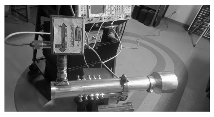
So again I replaced the TX probe SMA connector to an N connector and began adjusting and testing.
