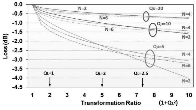
Figure 11 Insertion loss vs transformation ratio and inductor Q
