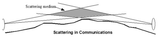
Figure 1. Over-the-horizon contacts made by radio amateurs usually involve scattering.
