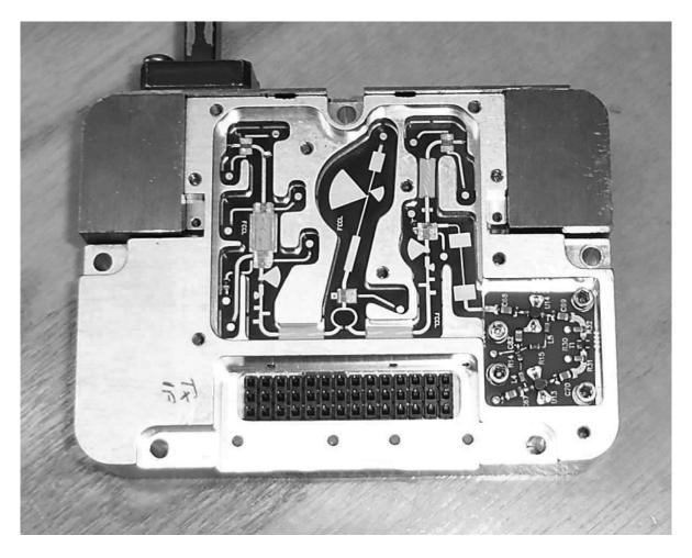
I was intrigued by a 'milli-meter transceiver' on ebay from 'rf-buy2008'. Described as a 'Signal Technology' unit, but with no frequency information. From the dimension of the waveguide hole I guessed at 40GHz. What I was hoping for was >40GHz, what I got was 37.4GHz – bother! The picture shows the business part of the unit, with the duplexor and waveguide power coupler removed.
