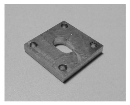
Figure 17 Waveguide Step Matching Transformer
