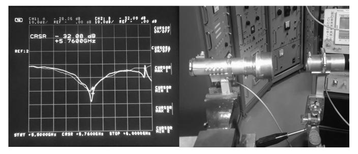
With the improved IMU launcher section mounted the whole feed was once again rechecked and tuned for best results. The TX probe Return Loss was about 28 dB and the Isolation test between the two probes came in around 32 dB. Very little changed now when the IMU was rotated around the feed pipe.
