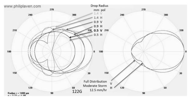
Figure 15. 122GHz plots of scattering. On left, three drop sizes in two polarizations. On the right, scattering with a drop size distribution as found in a moderate rain storm of 12.5mm/hr (1/2 inch/hr).
