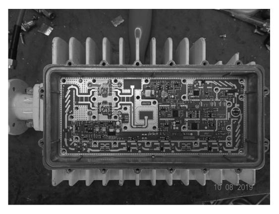
The 2 off Phased Eudyna MMIC's are top left. There are 4 off PCB Pads for DC Supply Rails. The two on the left are the -Vgg Bias Rails whilst the 2 on the right are the +VDD Rails.
