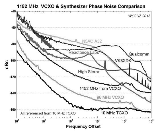
Figure 1 - Synthesizer Phase Noise measurements from 2012 and 2013
