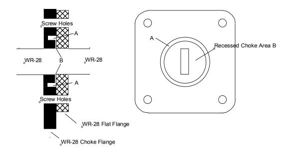
Figure 1. Cross sectional view
