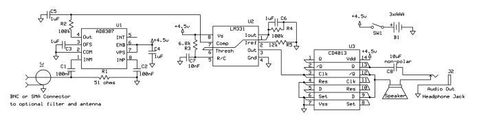
Figure 3 500 MHz version of Audible Field Strength Meter using AD8307
