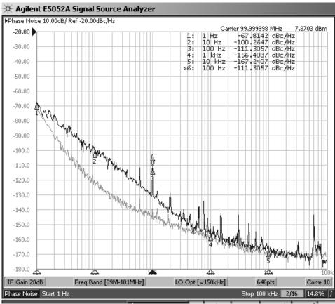
008 Plot 1 10MHz OCXO Reference Oscillator and 100MHz OCXO Reference Oscillator Compared Phase Noise
