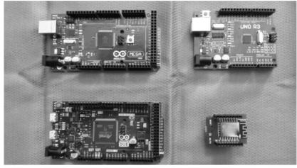
Figure 4 Example Arduino/WEMOS Controllers
