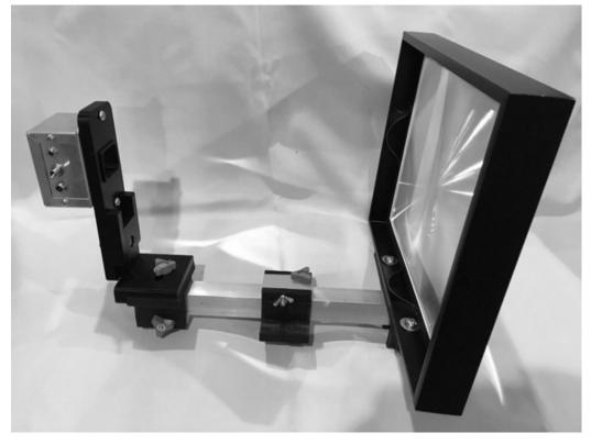
From left to right; Optical receiver, K0XL 3-axis receiver mount, tripod mount with rail tensioner, and the fresnel lens mount, all mounted on a 1-inch square aluminum boom
