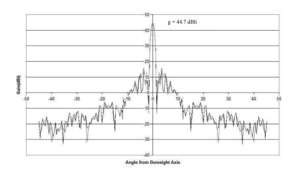
The computed gain shows an illumination efficiency of 72% for S-Band and 70% for X-Band. Sidelobes are down more than 20 dB below the main beam.
