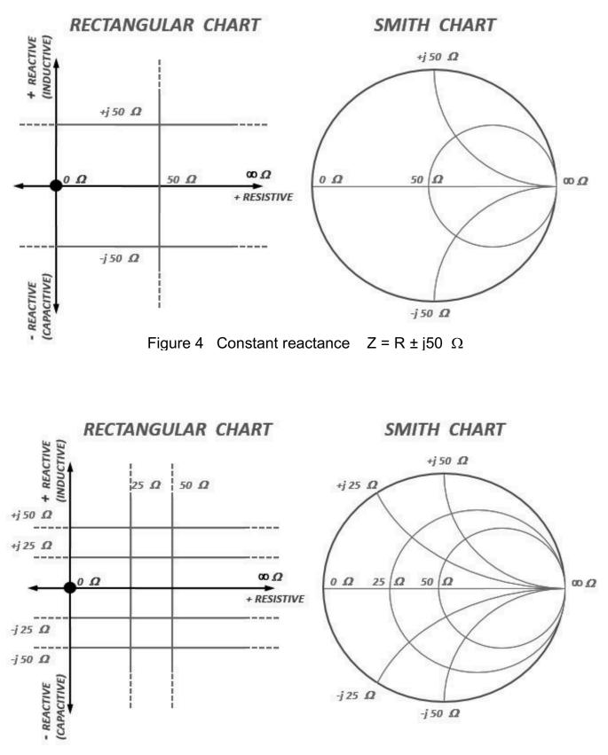
Figure 5 More constant R and X lines produce the impedance view chart
