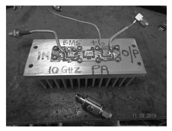
The final result can be seen here in this Photo of a single Amplifier.
