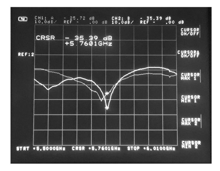
This feed with the longer copper pipe waveguide and using the ten brass bolts for the Circular Polarization was at first a battle to get adjusted and tuned.
