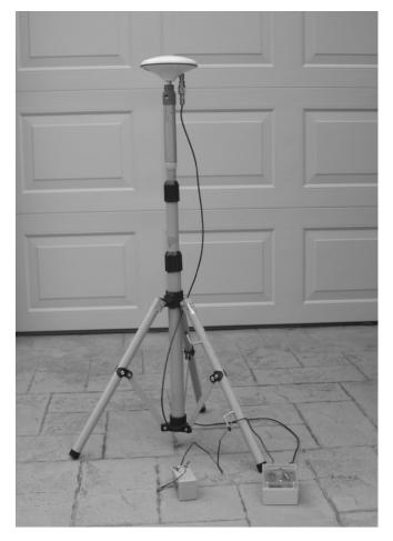
Fig 7: Base antenna with u-blox evaluation board in weather proof box and separate battery
