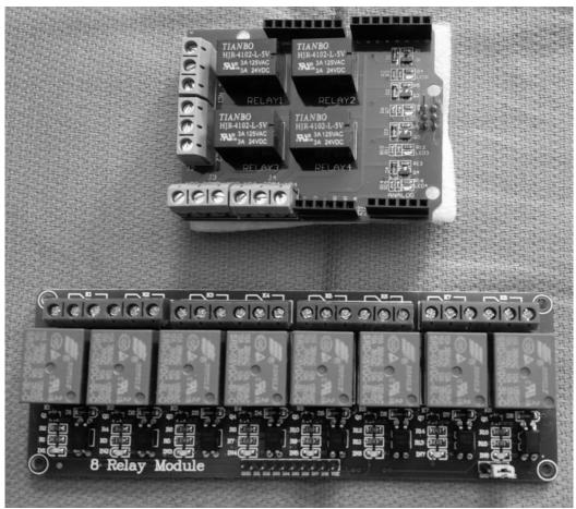
Figure 6 Arduino Compatible Relay Boards
