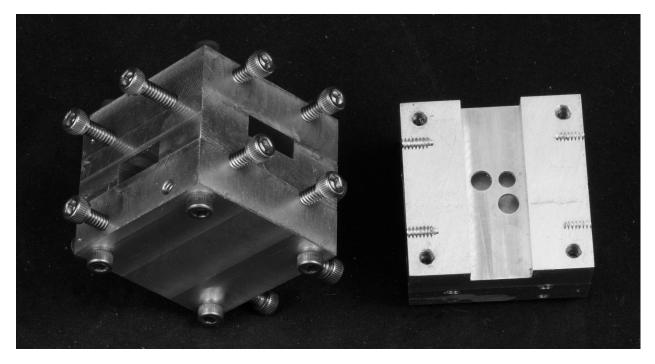
Figure 6 – Machined round hole cross-guide coupler for 24 GHz in WR-42 waveguide
