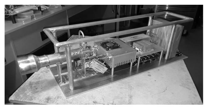
This is a pix of the new complete 6 CM feed assembly ready to be placed on the dish feed mounting shelf. It's controlled and monitored by a PIC microprocessor in the back box, and uses a Kuhnes transvertor and receive preamp. Lots of testing of the circuits was done to get to this point of the project.
