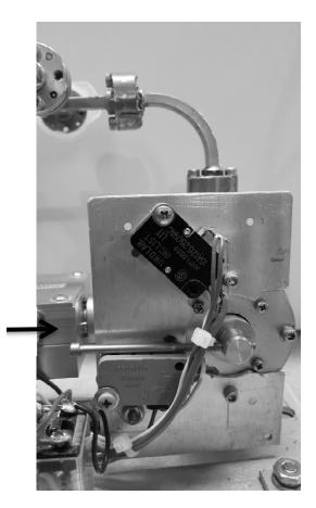
Figure 3 Waveguide Relay in the Receive position
