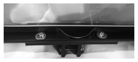
I use <sup>1</sup>/<sub>4</sub> inch hardware to secure the frame to the mount, bolts, washers, and lock nuts. It creates a solid platform for holding the lens as well as making it easy to change the lens size.
