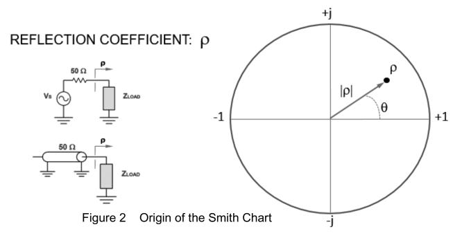
In other words, ALL possible passive reflection coefficients are contained inside this circular region. Equivalently, ALL possible passive load impedances are representable by points contained inside this circular region.
