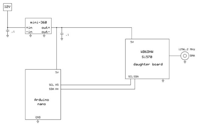
**Figure 2.** A simple beacon signal source using an Arduino (UNO, Nano, etc.) to write the frequencydetermining registers of a Si570 programmable oscillator upon startup. The daughter board contains a Si570, a 3.3-V regulator, several pull-up resistors, and a level shifter to communicate I2C data from the 5-V Arduino to the 3.3-V Si570.
