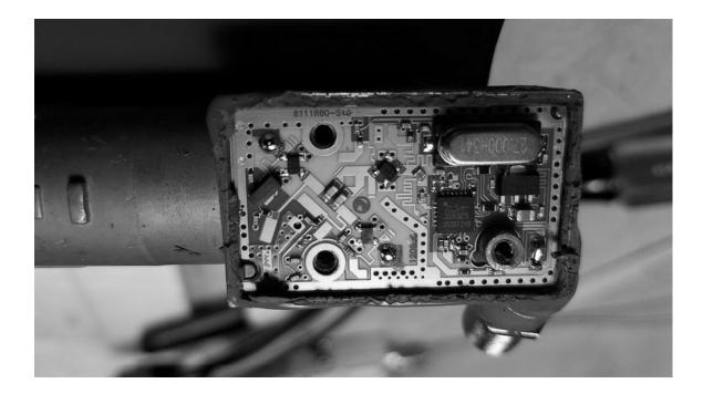
You can clearly see the modification. TCXO input, 6v from the regulator and a ground contact. Just use very small wire and RTV them down so they don't move.
