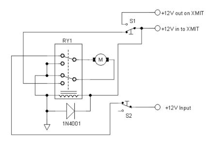
Figure 5 Schematic diagram of relay switching circuit
