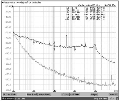
0010 Comparison of a Wenzel 10MHz free running OCXO vs 10MHz GPS phase noise
