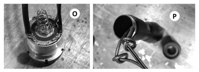
When you are happy that everything is working as expected it's time to reassemble your new lightwave transmitter. Start by press fitting the board back into the LED assembly (O).
