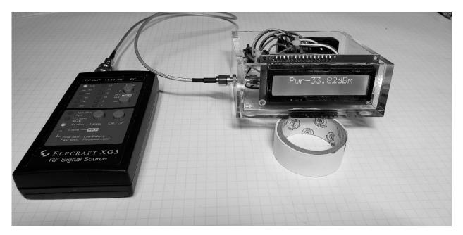
Figure 3. The power meter in operation.
