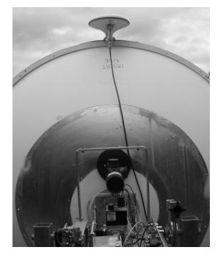
Fig 6: Rover antenna mounted on dish directly above rifle scope
