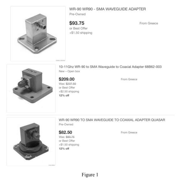
When you make a purchase of one of these you are sometimes surprised to find the part is advertised as WR90 but the dimensions of the waveguide or the mounting holes do not match other WR90 waveguide pieces you have. In addition you have no idea what the real performance of the converter is until you test the device.
