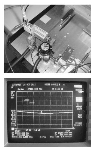
Noise figure measurement with a HP346C K01 source. For 47GHz read 27GHz as the 8593E analyser allows a max. frequency offset of 30GHz!
