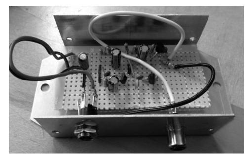
This is the finished receiver in the enclosure. I built it in a Hammond Manufacturing aluminum box #1411FBCU. The opening is for the BPW34 detector. It is connected "in the air" to the gate of the JFET. This minimizes the capacitance and increases the sensitivity of the detector. On top are the connectors for power (left) and audio-out (right).
