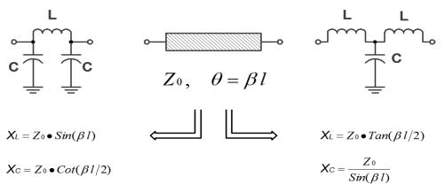
Figure 12 LC representation of a short transmission line
