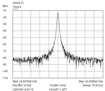
The plot shows the module being used as a harmonic mixer on an Advantest R3271 spectrum analyser. Although the analyser will work at 24GHz, in this case it is in external mixer mode. A single connection is used between the analyser and 'Det' SMA on the module. LO drive and IF input are on one coax, as the analyser contains an internal duplexor. Trying to use LO on the 'mlt' input, and using 'det' as an IF output did not work.
