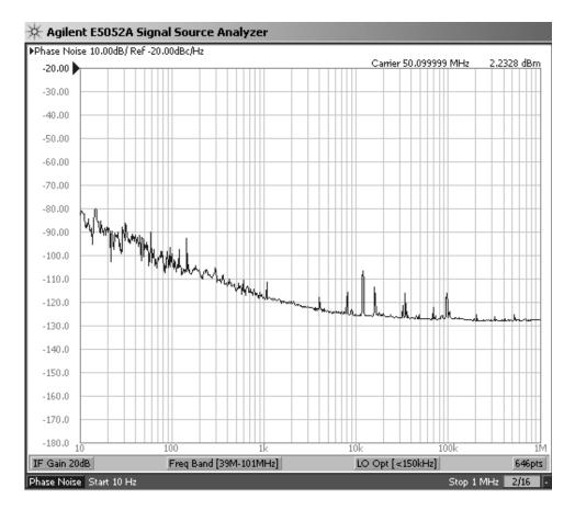
ICOM-7300 Transceiver 10Hz to 1MHz phase noise 50.1MHz transmit frequency set to 20% power output with a 40dB power attenuator in line. These transceivers offer great performance and very clean signals as compared to the early radio synthesizers. Its good to keep in mind that this clean transmitter and receiver will be degraded if you mix these signals in a transverter with poor phase noise performance. Your mixed signals will take on the characteristics of the poor synthesizers phase noise.
