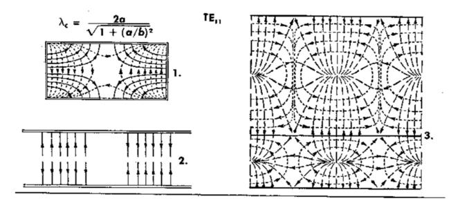
Figure 3 TE<sub>11</sub> Propagation Mode (Cut-off Frequency 47.2 GHz)
