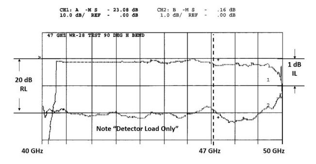
Figure 11 Rigid Waveguide 90 degree H Plane bend
