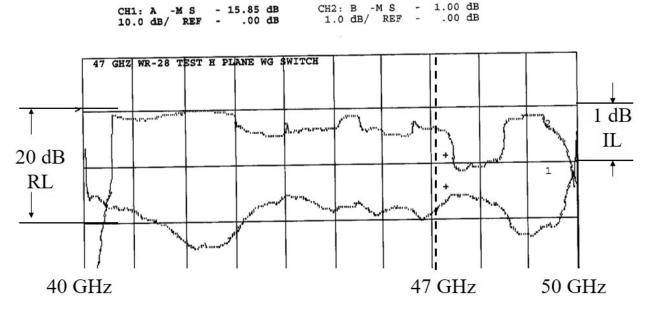
Figure 19 Waveline 1078-H H plane Waveguide Switch
