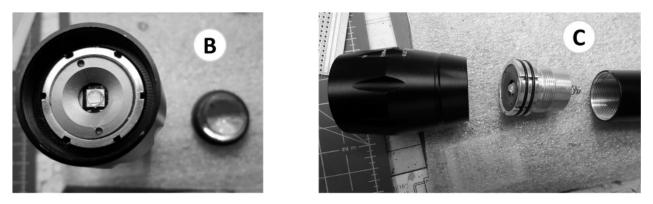
Remove the copper colored (inner ring) LED retaining ring. There is a clear spacer under the retaining ring, keep this as it protects the LED connections from shorting out. The LED and heat sink are now exposed. Unsolder the red (+) and blue (-) wires from the LED base (D). Clean off the LED assembly base and add new heat sink compound and add your new IR or red LED and solder it in place (E).
