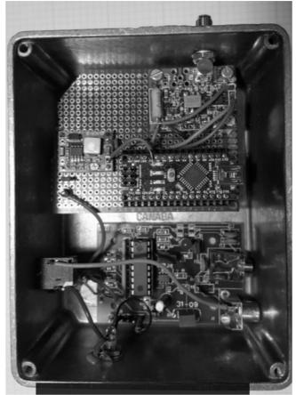
**Figure 6.** The signal source is enclosed with a KT-4 beacon keyer in a Hammond box with a 2.5 mm jack that brings in 12V, and a 3.5 mm stereo jack that brings in an amplifier sample voltage and the keying line. The RF is brought out via the daughterboard SMA and an RCA jack is used for external metering of the amplifier sample voltage.
