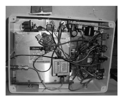
To allow for CW keying, I used an inline 'modulator' which switches the synth. output. FM was very last minute. I wanted some audio amplification and limiting. The only thing I found was a compressor chip, that I had never got around to using. This was stuck on the synth. and bias provided for an electret microphone.
