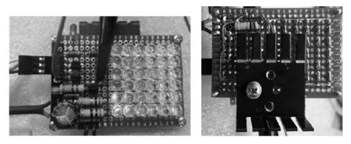
Front side of 36 LED Transmitter with current driver, back of board with FET heat sink view
