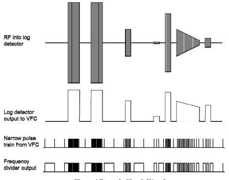
Figure 4 Example Circuit Waveforms
