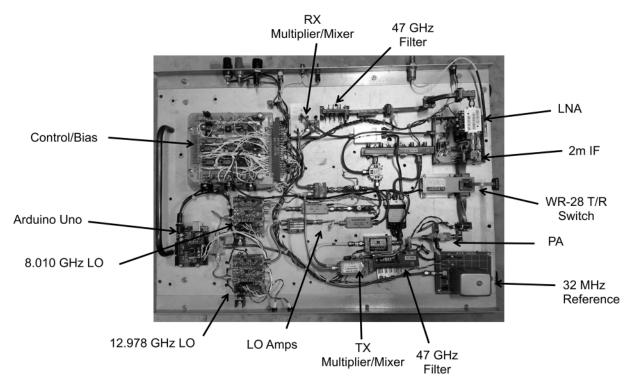
Figure 3 AA5C 47 GHz Transverter
