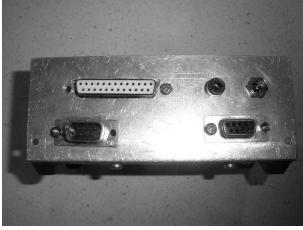
Figure 4 Rear Panel view of the decoder
