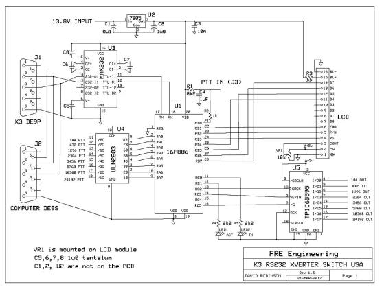
Figure 1 Circuit diagram
