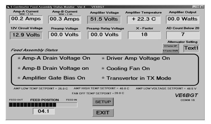
Amplifier Circuit and Voltage Points in Transmit Mode, Keyed Only.
