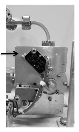
Figure 4 Waveguide Relay in the Transmit position
