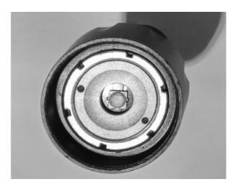
Figure 3 Removal of LED Assembly
