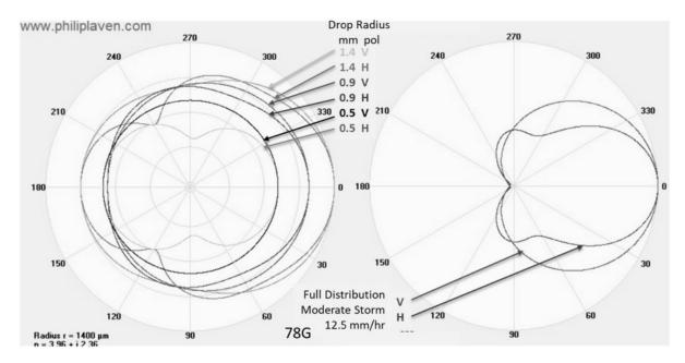
Figure 14. 78GHz plots of scattering. On left, three drop sizes in two polarizations. On the right, scattering with a drop size distribution as found in a moderate rain storm of 12.5mm/hr (1/2 inch/hr).
