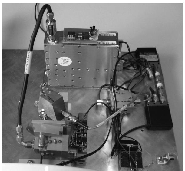
The synthesiser is at the top of the picture, with it's PIC loader board on top. Firmware is from Dave G4FRE, and is available on his website. In the foreground is a X3 tuned multiplier, which drives a mm-tech 23 -36GHz WR-28 amplifier. It was the appearance
