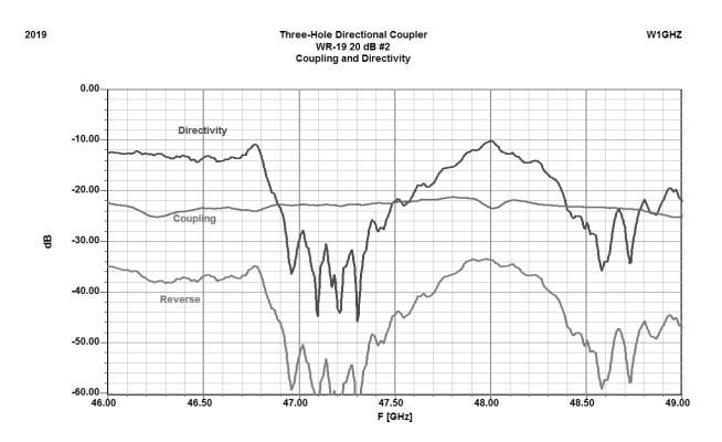
Figure 11 - Measured performance of round hole cross-guide 20 dB directional coupler for 47 GHz in WR-19 waveguide
