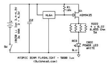
Schematic for the board in the Atomic Beam Flashlight
