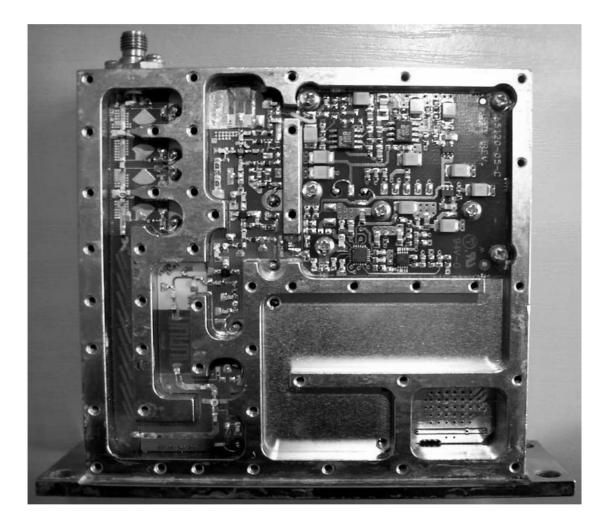
RF side of the synthesiser showing the hairpin and stripline filters at the bottom left. Some useful frequencies CDFSL-1201 (11.2 – 12.0GHz)
