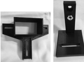
Vertical slider w/light shield Horizontal slider
