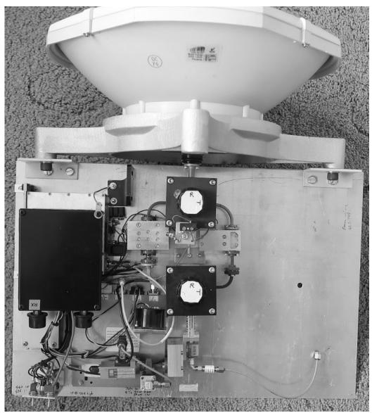
How the transverter looks in 2019, with 30cm dish, and two WG switches.
