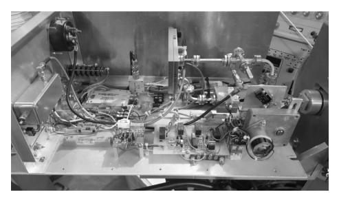
Figure 1 Completed 76GHz Transverter
