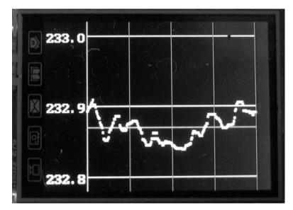
Fig 4: This is a graphical display of the indicated bearing over last 20 minutes. The green line shows the average reading which in this case is around 232.87 degrees with a variation shown by the white graph to be well within +/- 0.1 degrees.
