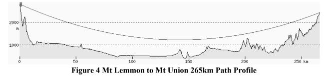
As mentioned earlier the ability to knife edge or go over the horizon is unknown as yet. A 280km hop exists from Mt Lemmon to Mt Harquahala which has some obstruction (~ 10 m or 35 ft). This hop was studied closely and the most optimistic path profile used the commercial software and is shown in Figure 5. Other similar slightly obstructed hops exist elsewhere that could be record breakers.
