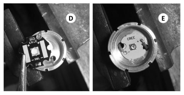
A word of caution is needed at this point. Depending on the LED you are using and the base it is mounted on, you may need to make a small modification to prevent shorting out the LED.
