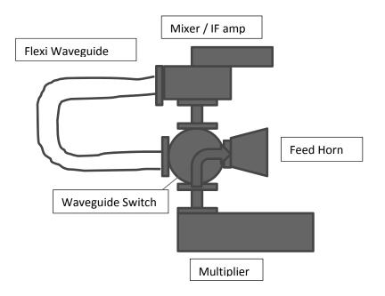
Waveguide Switch in Transmit position.
