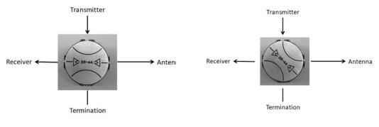
Figure 1 Waveguide Relay in Receive Position
