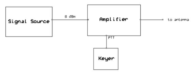
Figure 1. A typical CW beacon consisting of a signal source, a keyer, and an amplifier.
