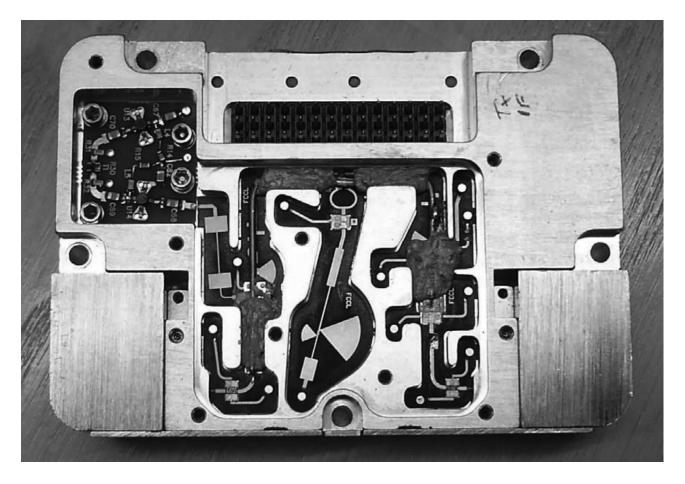
I used miniature coax that was to hand, as it was likely to propagate the high frequency and give some attenuation between LNA and driver. I soldered the inner on to the track at the LNA end, and used liberal amounts of silver epoxy to connect the outer. This I found I needed to cure, so I put it in the oven at 100 deg.C for an hour, which seamed to do the trick. At the Tx filter end, I bent the inner down and used silver paint to make the connection.
