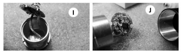
This is the LED control board (J). Part numbers may be different from the schematic; we found part ids were different between shipments. Thankfully it isn't a complicated schematic and the board is easily modified.
