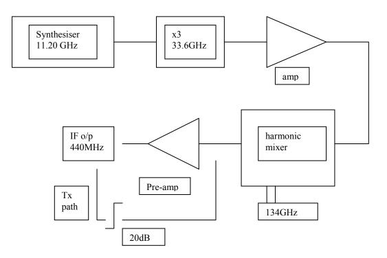
Simplified 134GHz transverter block diagram
