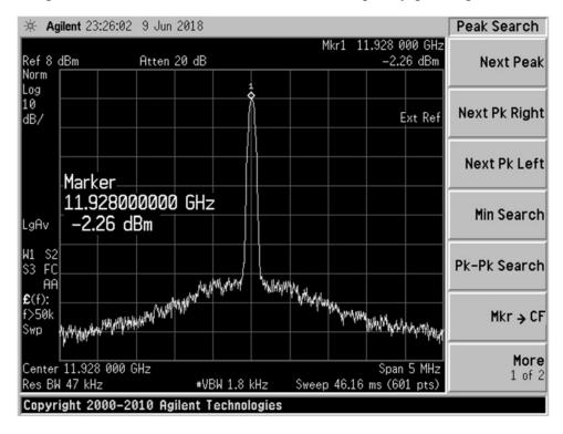
SCR514 Reprogrammed to generate a 11928MHz LO which can be used with a subharmonic mixer to make a 24GHz transverter. The LO operates at ½ frequency and is doubled in the subharmonic mixer, this alleviates the need to double the LO frequency before the mixer. Keep in mind that doubling the LO frequency in the subharmonic mixer will degrade the phase noise by 6dB from that shown on the plot.
