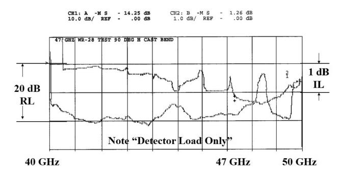
Figure 13 Cast Elbow H plane Bend
