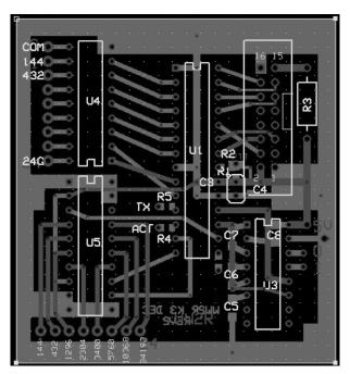
Figure 2 PCB Overlay
