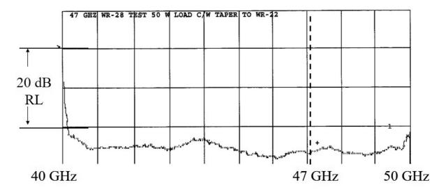
Figure 16 50 W Load with Taper Transition to WR-22
