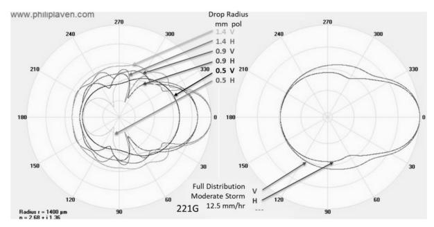
Figure 17. 241GHz plots of scattering. On left, three drop sizes in two polarizations. On the right, scattering with a drop size distribution as found in a moderate rain storm of 12.5mm/hr (1/2 inch/hr).
