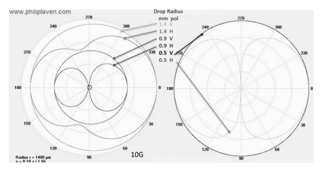
Figure 10. All these plots assume that the incoming EM wave is from the left. On 10 GHz it was impossible to see the shape from the smallest drop size on the same plot as the larger, but on all the others they "fit". In this figure the smallest drop size plot is a small circle on the left plot, but is expanded to an entire plot by itself on the right.
