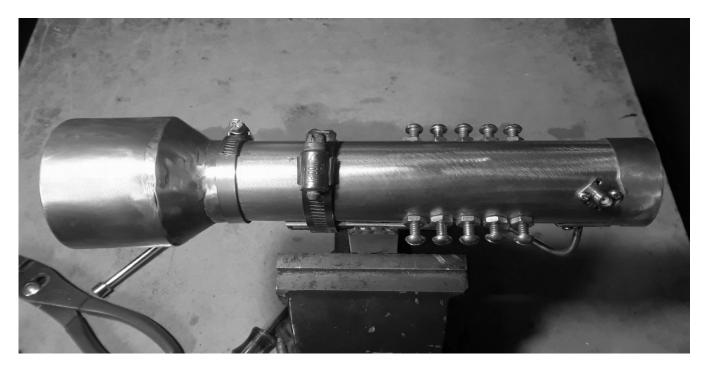
The New Constructed Short Feed, TX Probe Using a SMA Connector
