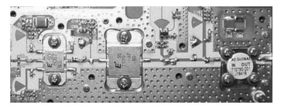
Power Amplifier mods for 2.7W Output. Driver FMM5057VF, PA FLM7179-4F,
