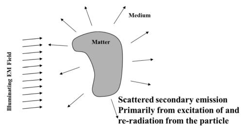
Figure 3. Particles re-radiate energy that enters them
