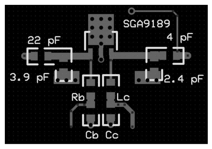
Figure 22 Overall SGA-9189 amplifier layout
