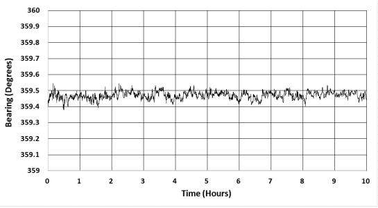
Fig 9: Results with Survey Grade antennas over a 5 metre baseline with a clear view of the sky.
