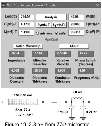
equivalent to a 2.8 nH inductor with 0.24 pF parasitic shunt capacitance at each end. This is representation is shown in Fig. 19.
