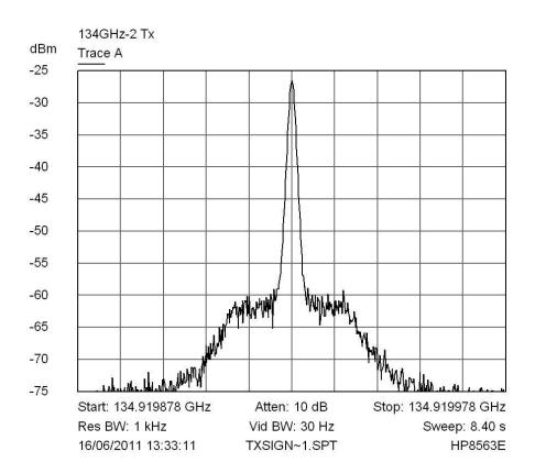
This is the Tx output spectrum of the second transverter. The true output power is greater than that shown as the mixer is calibrated with a 13GHz LO, and the spectrum analyser LO output is being used to drive it (around 4GHz).
