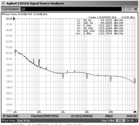
005 Plot 3 1152MHz LO for 1296MHz converter phase noise
