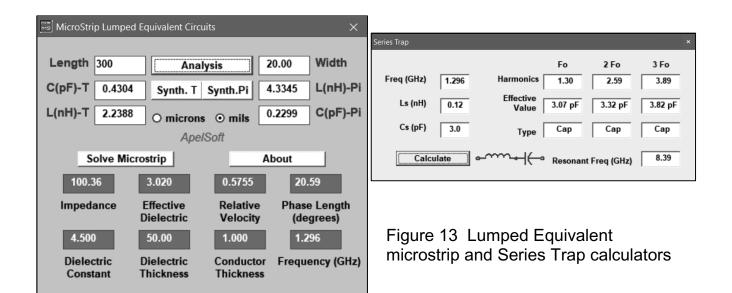
Before we work through a design example, it is worth pointing out that a useful estimate of the self-inductance of various surface-mount chips can be made with the microstrip lumped equivalent calculator by loading the package footprint length and width. These results, over a
