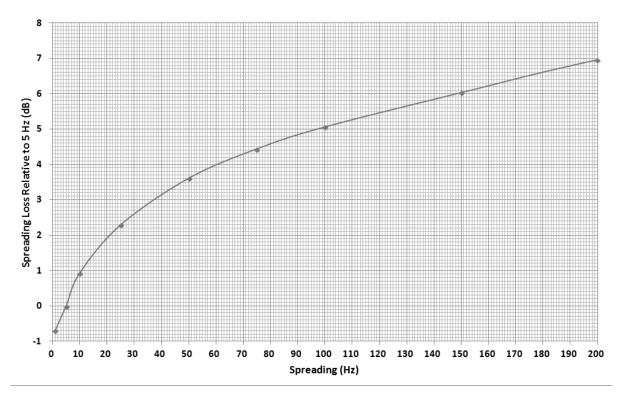
Fig 1: Libration Spreading Loss derives from DUBUS Paper by VK7MO and G3WDG<sup>(1)</sup>
