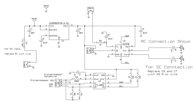
**Figure 4.** A Si570 daughter board from WB6DHW. If a 3.3-V Arduino is used, then the level shifter U3 would not be necessary.
