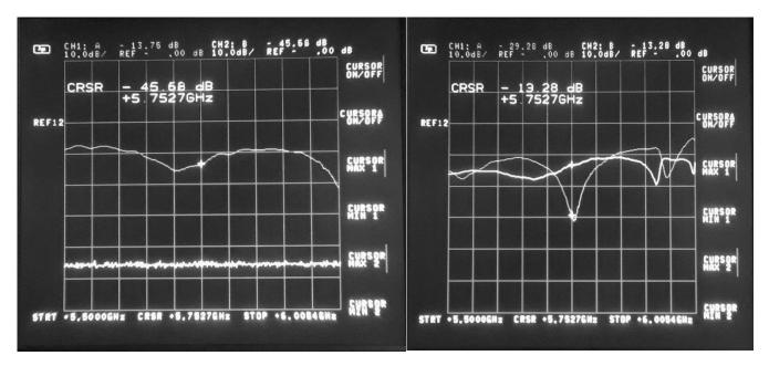
The left pix is trying to adjust the probe only using different thickness of wire. Then on the right pix the IMU launcher and back plate being adjusted for a Return Loss of 29 dB. Isolation again between receive and transmit probes is poor at only around 13 dB. Next was to try the CP bolt adjustment.
