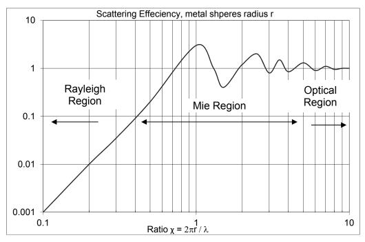
Figure 4. Scattering efficiencies vs. frequency for spheres. Various materials will reach the resonance region at slightly different ratios but the general form of this function is the same regardless of the material.
