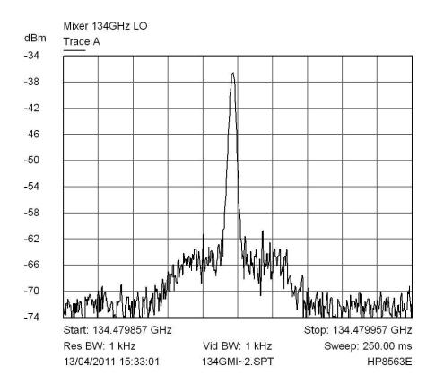
The spectrum plot of the LO signal at 134.480GHz. This using the internal 10MHz reference in the synthesiser. I am staggered how clean and stable the signal is! However since that first QSO, I found that the signal was not as clean when on battery. I was using a series diode in the supply. When the supply dropped below 11.4V the LO moved frequency and spurs were produced. Something I have never noticed at fundamental! It is fine on 12.0V.
