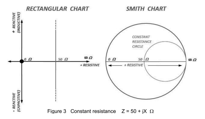
Impedance is a complex number with a real part and an imaginary part: Z = R + jX. Impedance represents a series connection of a resistor and a reactance. A positive reactance is inductive and a negative reactance is capacitive. Constant real lines (resistances) become circles on the Smith Chart. Note also that the positive real axis from the rectangular chart maps into the horizontal line that divides the Smith Chart into upper and lower halves.
