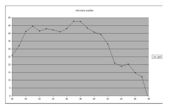
The response shows gain in dB on the vertical scale, against frequency along the bottom in GHz.
