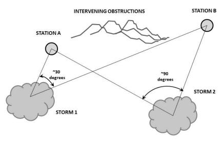
Figure 9. An example Situation. The two stations are much more likely to communicate via strom1 than storm 2 because storm 2 presents a 90 degree angle.
