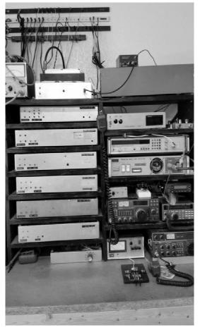
Figure 2 AA5C Microwave Transverters
