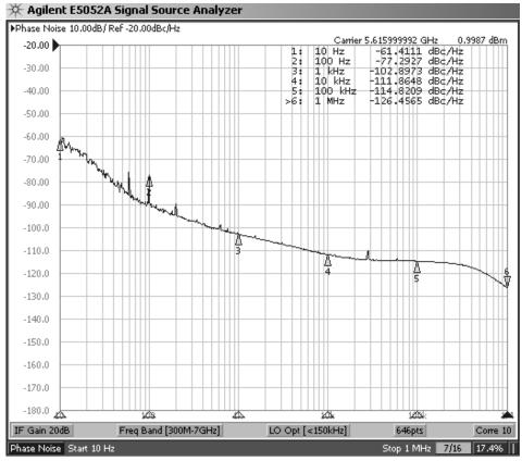
004 Plot 4 5616MHz LO for use with a 5760MHz transverter phase noise plot
