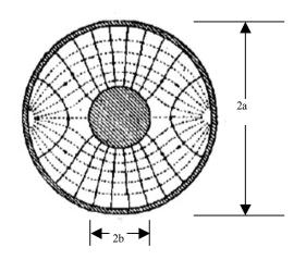
Figure 4. Electro-magnetic fields associated with TE<sub>1,1</sub> mode in coaxial waveguide
