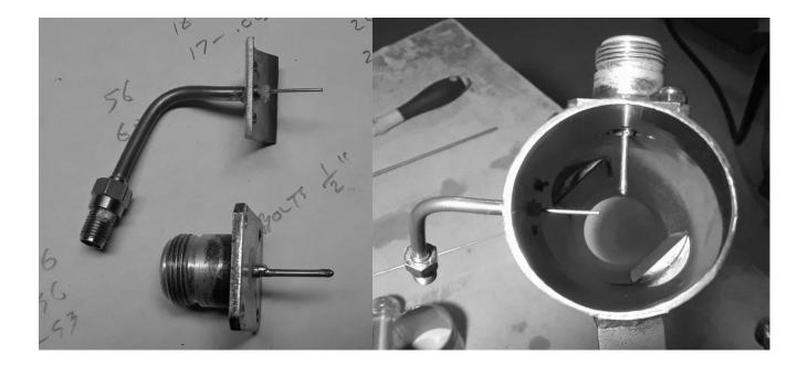
I then wanted to convert the feed over to an N connector for the TX probe and a custom rigid line connector for the RX probe. This RX probe line hooks directly to the SMA Isolation relay.
