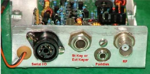
My rear panel contains a DIN connector that I use for my serial connections where I can change to various SoftRocks I use, without having to change cables on the back of the computer. The "key common" must be above ground ,so both the paddle connector (1/8" stereo connector) and the straight key/keyer connectors are isolated from chassis ground I did that with a piece of glass circuit board. As long as I was isolating things from ground, I
