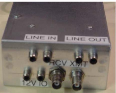
BNCs for 10M rcv and xmit RCAs for line input, output, +12V, and PTT to RS-232
