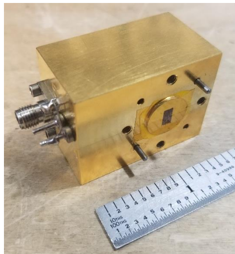
WA1MBA X4 47 GHz Multiplier (11776 MHz X4 = 47088 MHz) W5LUA AJWard 3/18/2024
