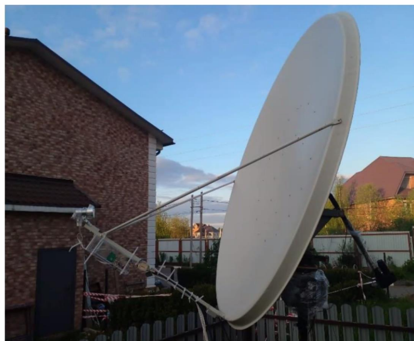
6.7 GHz methanol line telescope. The dish and downconverter outside, IF \approx 969 MHz.
