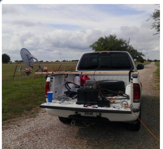
18 inch offset fed dish 400 mW Qualcom PA Double balanced mixer with no RF amplifier on receive
