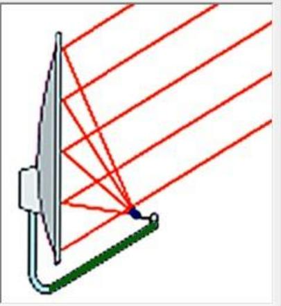
This program does calculations for oval-shaped offset-fed parabolic reflectors. This routine uses a curve-fitting algorithm to find the focal point and tilt angle for aiming the dish.
