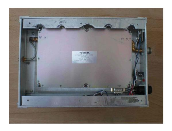
1mW input 50W output 12.6V @ 16A
